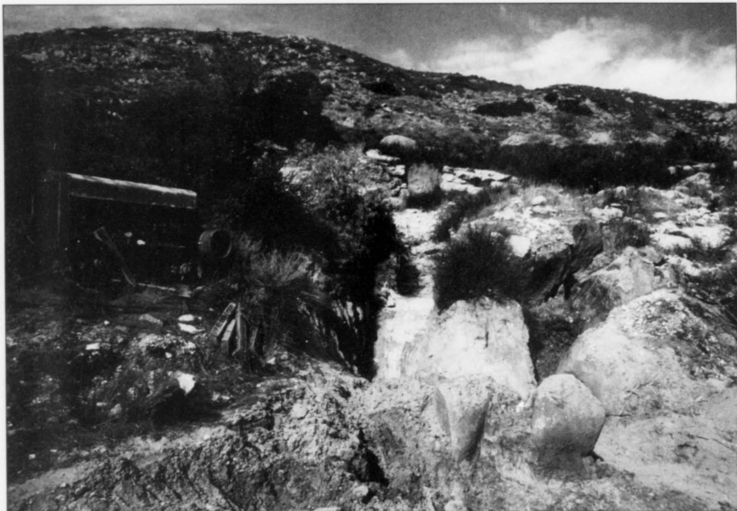
Figure 71. Surface workings on the main topaz-bearing dike at the Little Three mine, Ramona district, 1996. Jesse Fisher photo.
