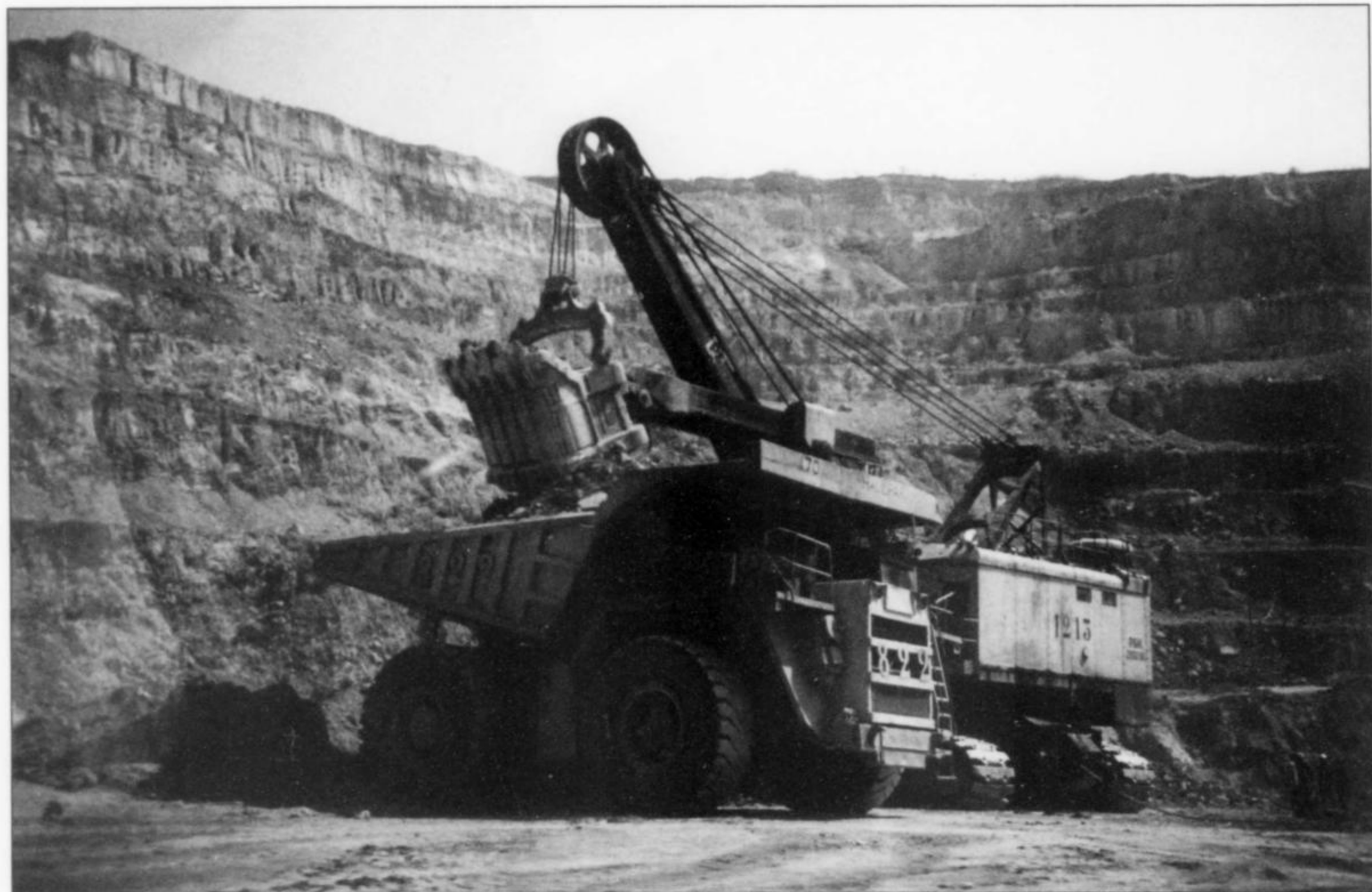
Figure 11. The KOV pit at Kolwezi. Copper ore is being loaded into a truck.
