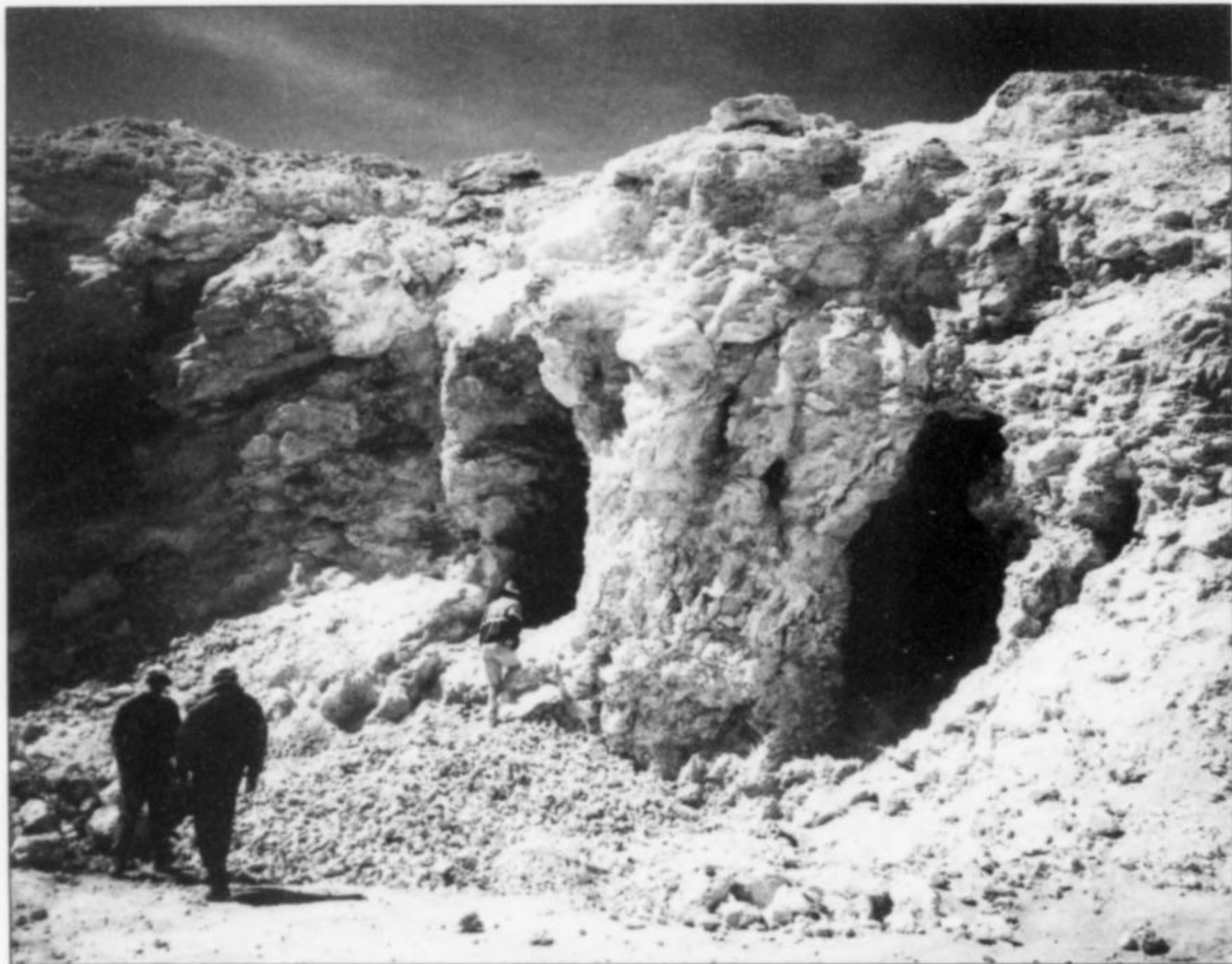
Figure 9. The face of one of the open cast pits at the El Desierto sulfur mine, showing mined-out fissures that were once lined with sulfur crystals. Rock Carrier photo.
