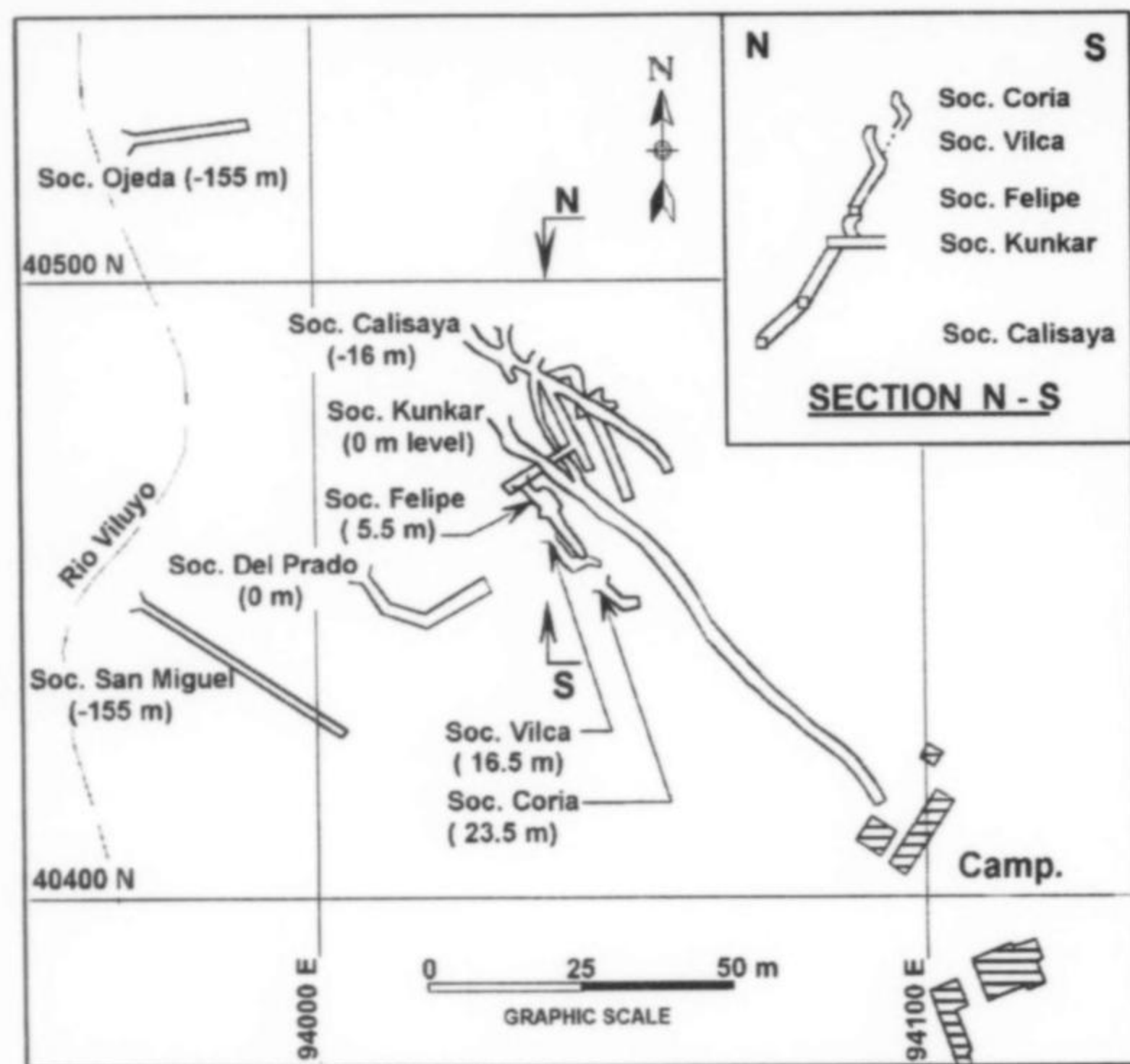
Figure 8. Plan of the old mine workings at Pacajake in 1935.
