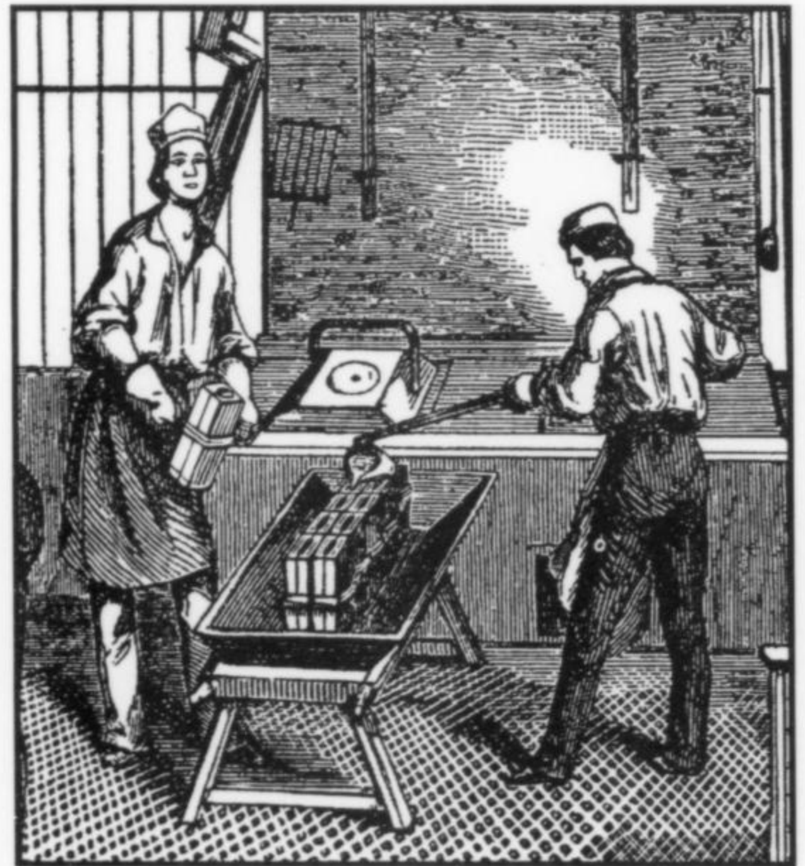
Figure 14. Foundrymen at an assay office in San Francisco are shown here pouring molten gold into ingot molds, after which the bars were cleaned, weighed, assayed and stamped before being returned to the miner or bank who brought in the gold.
