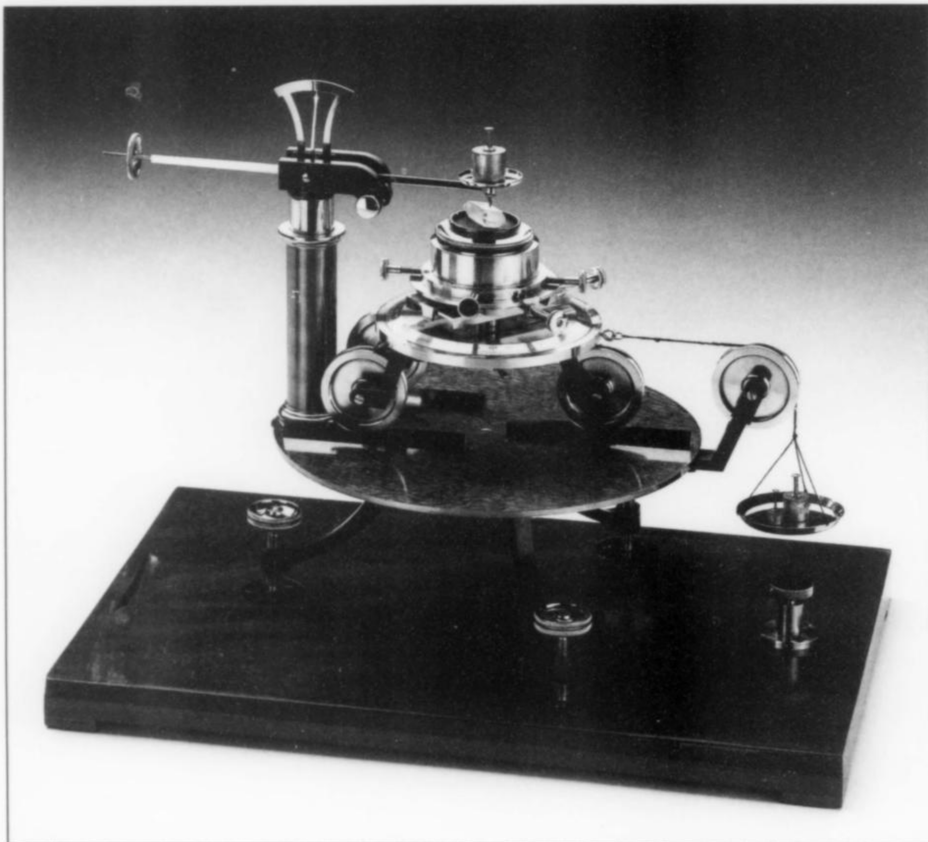
Figure 6. Scratch sclerometer with rolling weight system by Grailich & Pekarek. Signed "Voigt & Hochgesang, Göttingen," 1896.
