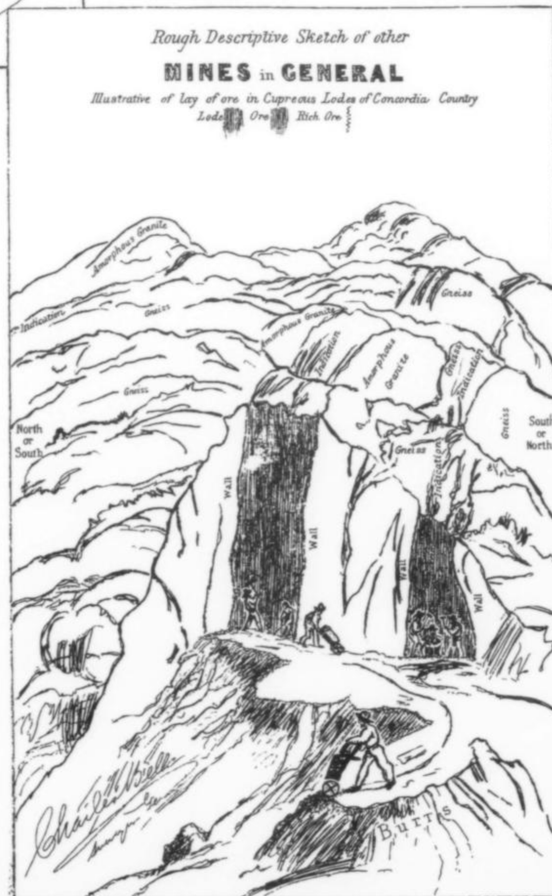
Figure 16. A sketch of the mines drawn by C. D. Bell. This illustrates the general granite-gneiss terrain and the steeply dipping orebodies. (From Bell, 1855.)
