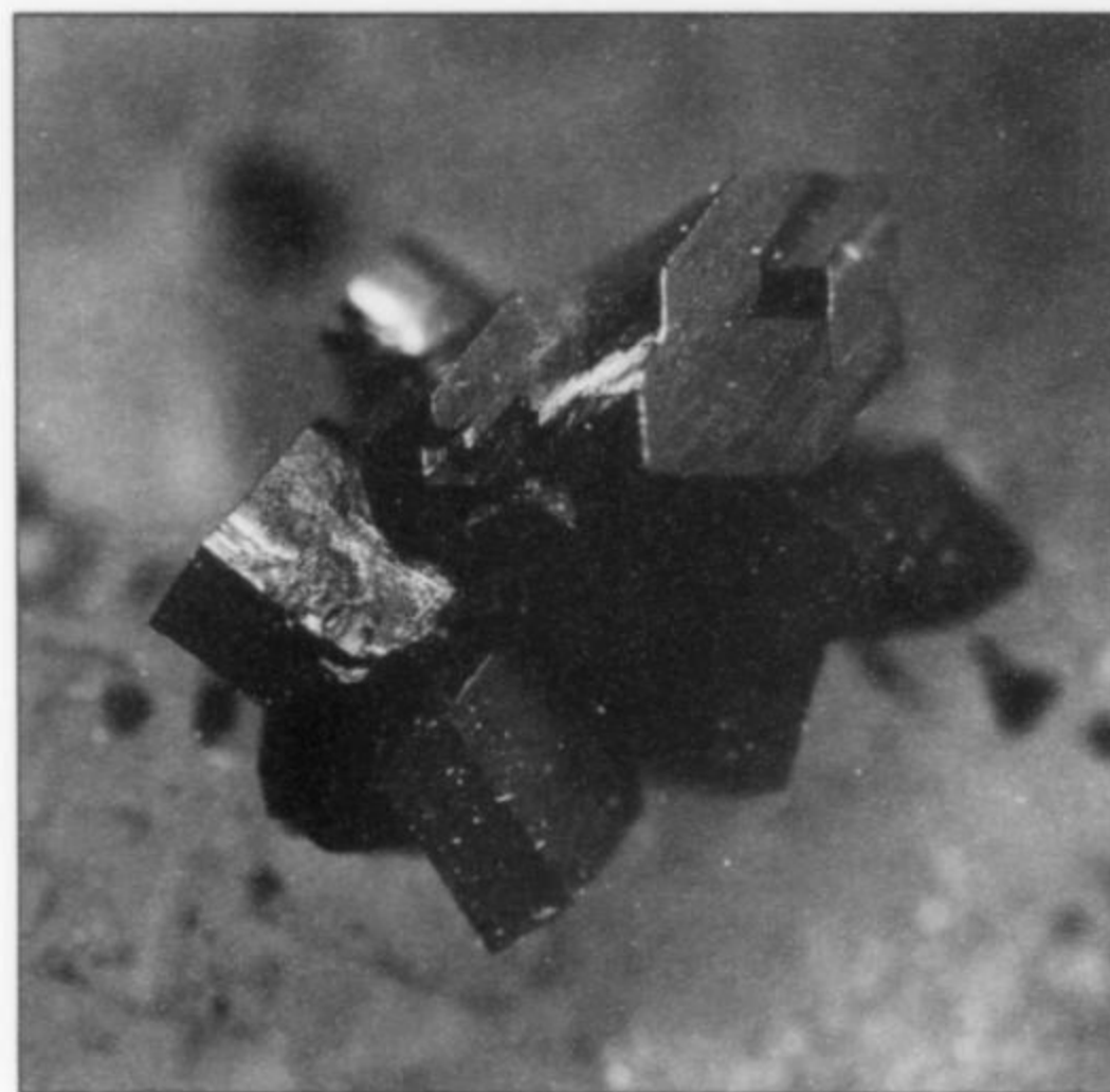
Figure 25. Enargite: close up of a 2-mm group of crystals on the specimen shown in Figure 28.
