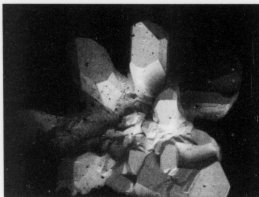
Figure 44. A divergent group of prismatic, black wattersite crystals, to 300 microns, in quartz cavity. Clear Creek mine, lower workings. Gail Dunning specimen and SEM photo.
