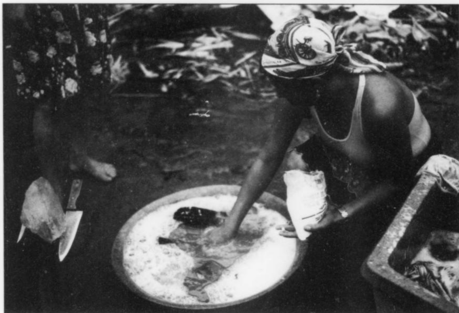
Figure 4. Washing of recently mined tourmaline and quartz crystals at the Santa Rosa mine. After washing, the crystals are scraped and further “cleaned” with a butcher knife—and thereby countless small crystals of rare accessory minerals are lost.
