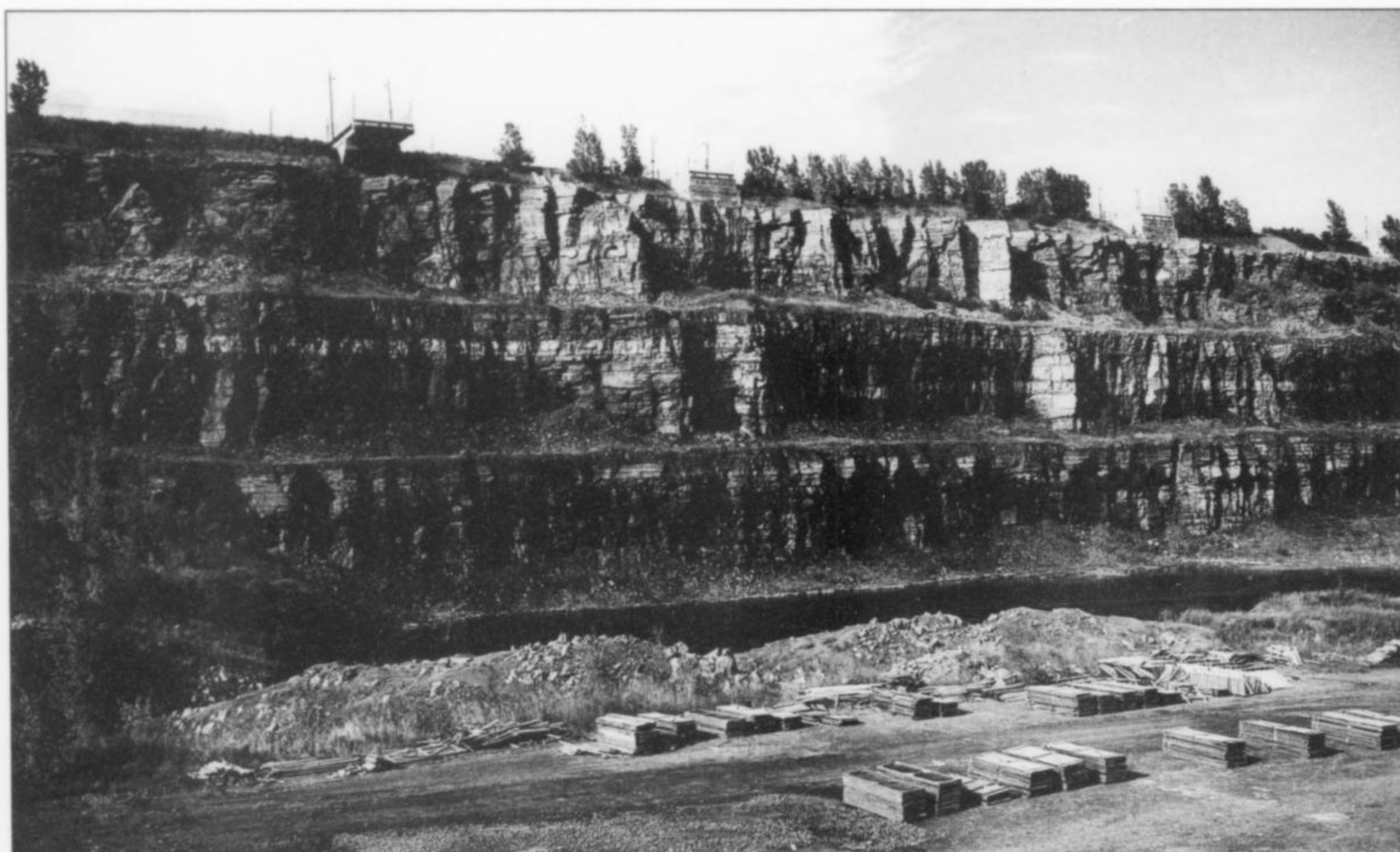
Figure 4. The northeast wall of the Francon quarry, with a view of the upper sill and the snow-dumping ramps. All three of the main levels and the upper sill are clearly visible. The water is from the previous winter's snowmelt. L. Horváth photo, 1992.
