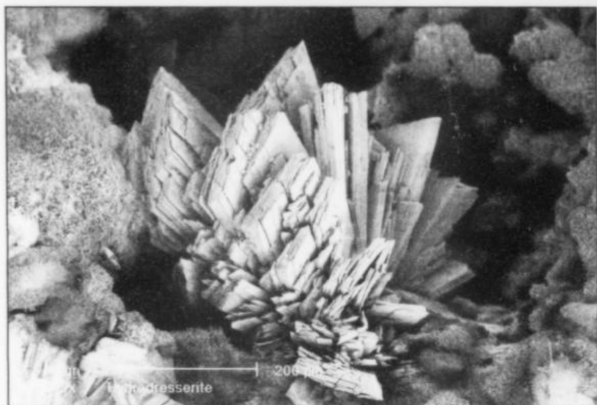
Figure 62. Radiating cluster of hydrodresserite microcrystals showing the triclinic morphology and the cleavage parallel to [010]. Horváth collection (no. 5234); R. Gault and L. Horváth SEM photo.
