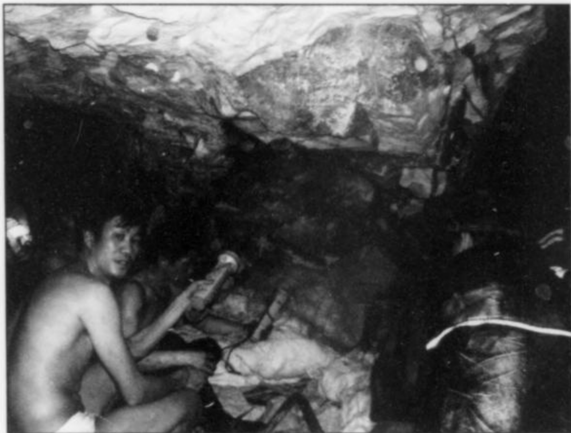
Figure 11. The pocket named "The Green Vault" extends in an upward direction. Over the course of a year, the rock was painstakingly chipped away from all sides to free the pocket in one enormous egg-shaped block. Ottens photo.
