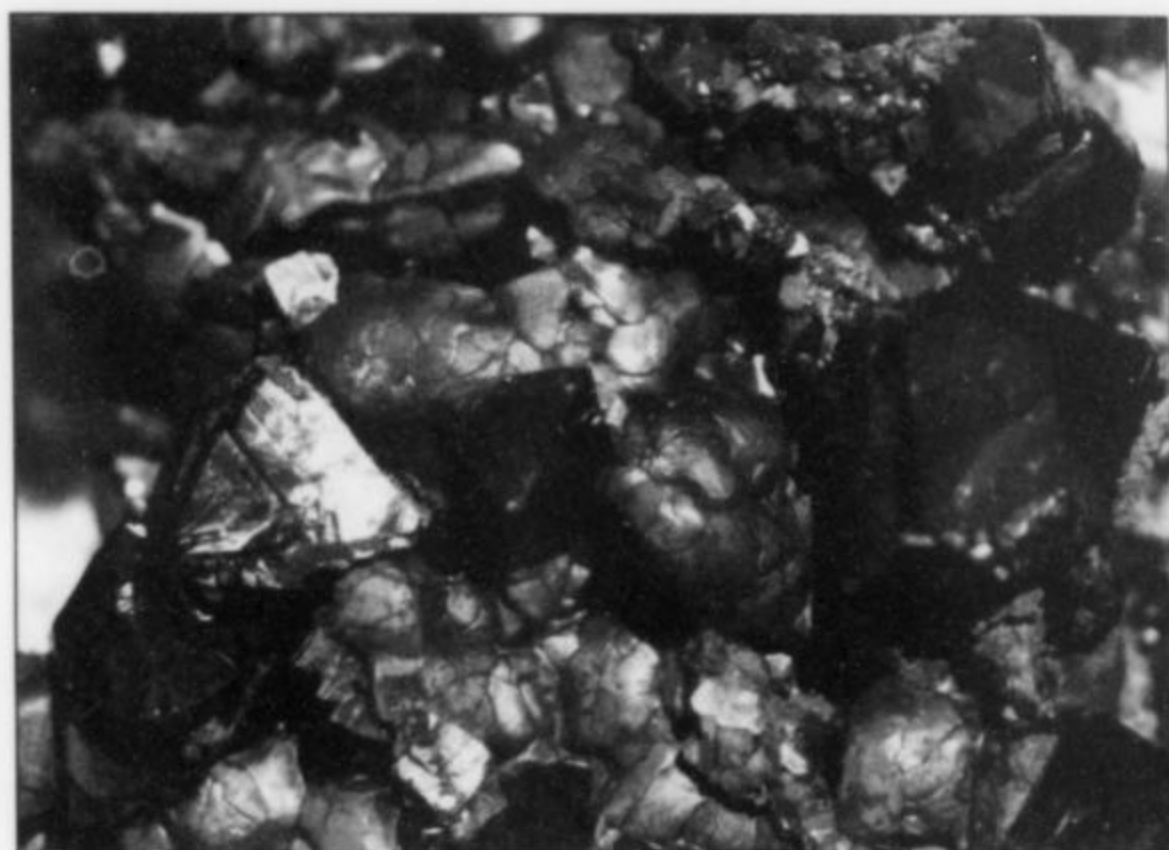
Figure 37. Rounded "flowed galena" in streams, with 1-cm sphalerite crystals and pyrite, from Trepča.
