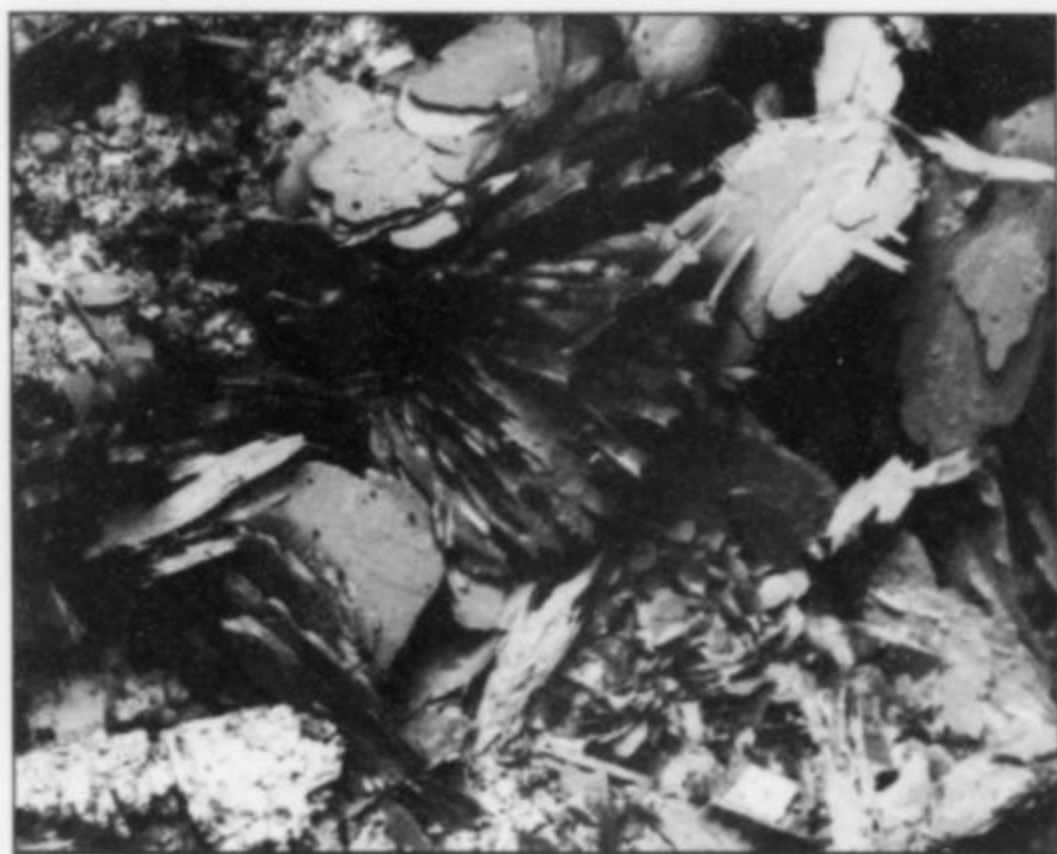
Figure 72. Scanning electron microscope photo of a fornacite specimen; field of view 0.7 mm. The typical tabular but pointed shape of the crystals is evident here. Bertrand Devouard REM photo.
