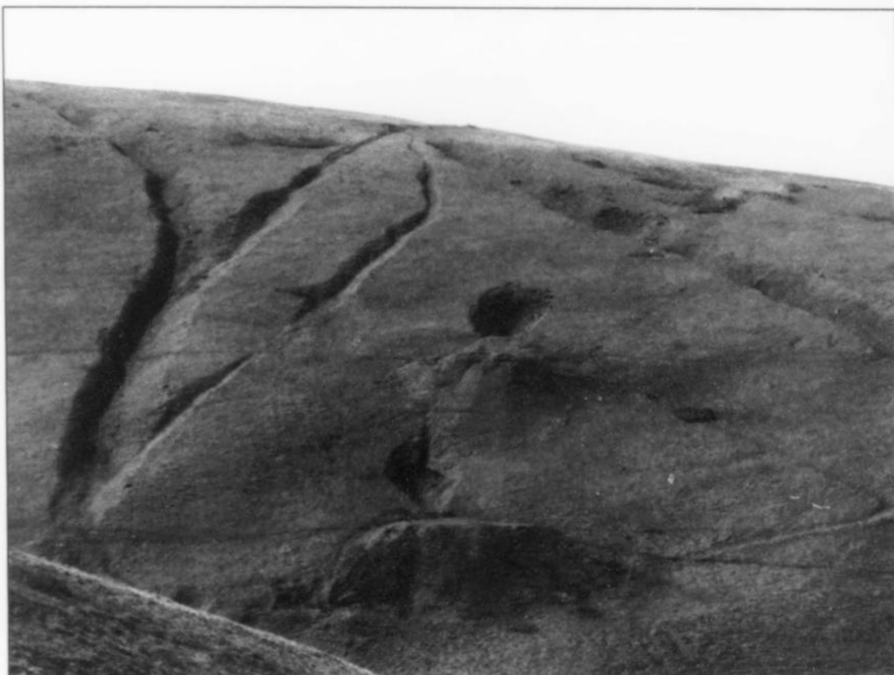
The Brae Fell mine. Note the "hushes" running down the hillside, created by miners who used pent-up water, released suddenly, to erode exploration trenches. Gordon Akitt photo.
