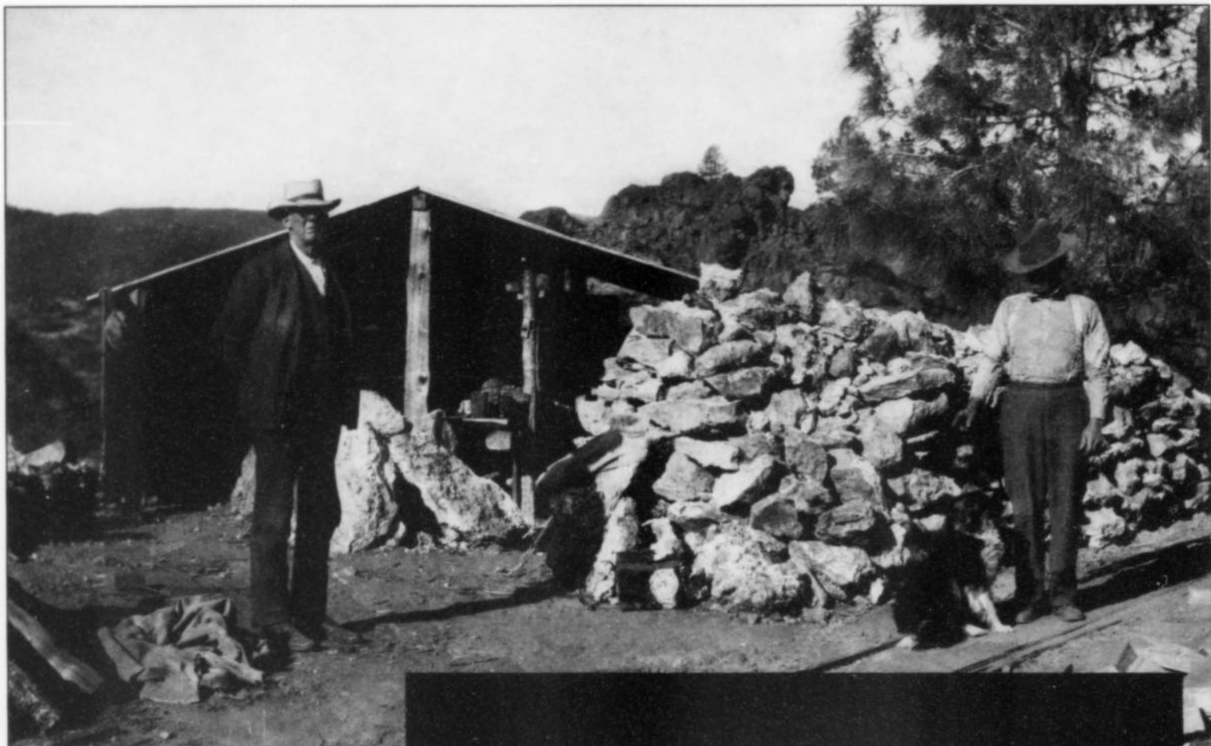
Figure 13. Dallas mine superintendent Thomas Hayes (left) and miner Emerson Humphries (and camp dog Fritz) in 1908, standing in front of a large stockpile of benitoite-containing natrolite vein material awaiting "processing," that is, manually breaking out the gemmy crystals to sell as gem rough. Only the non-gemmy crystals were saved for sale as specimens via mineral dealer Robert M. Wilke. (Courtesy Collector's Edge Minerals .)
