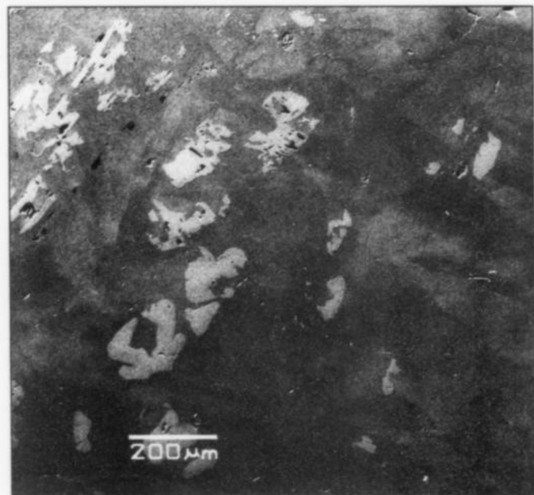
Figure 15. SEM backscatter image of olmiite near the rim of specimen no. 8280b, showing brighter areas with higher Mn content.
