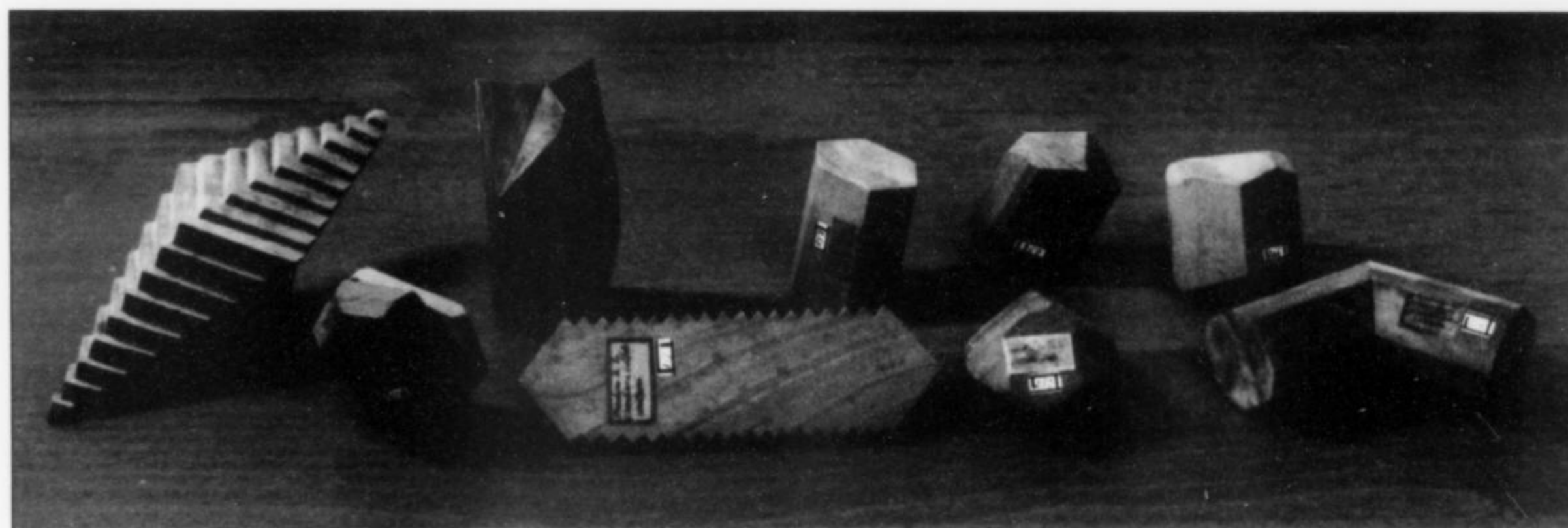
Figure 4. Some Haüy crystal models: two decrements, three twins (one of which is a pivoting model) and four models of different classes. Authors collection.
