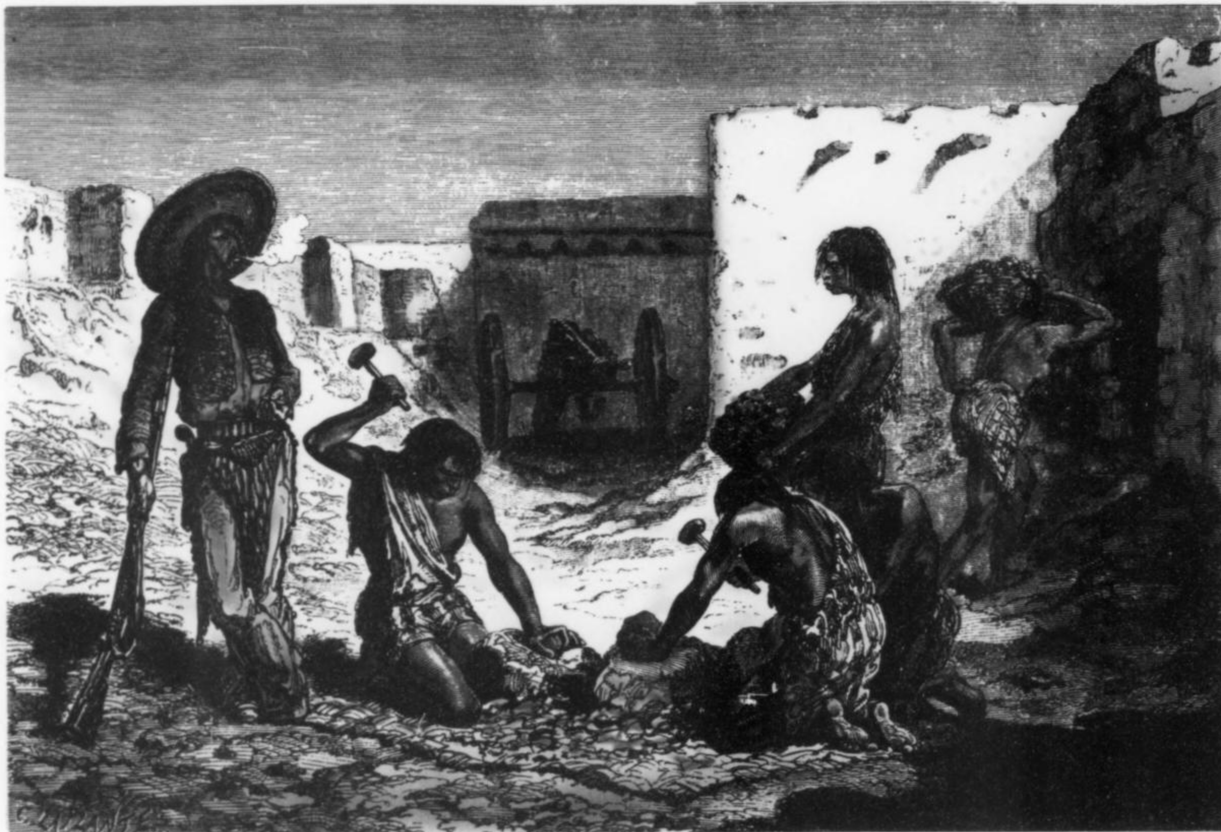
Figure 17. Indian prisoners employed as forced labor, cobbing out silver ore at a mine in Chihuahua; from Louis Simonin's Life Underground, or Mines and Miners (1869).
