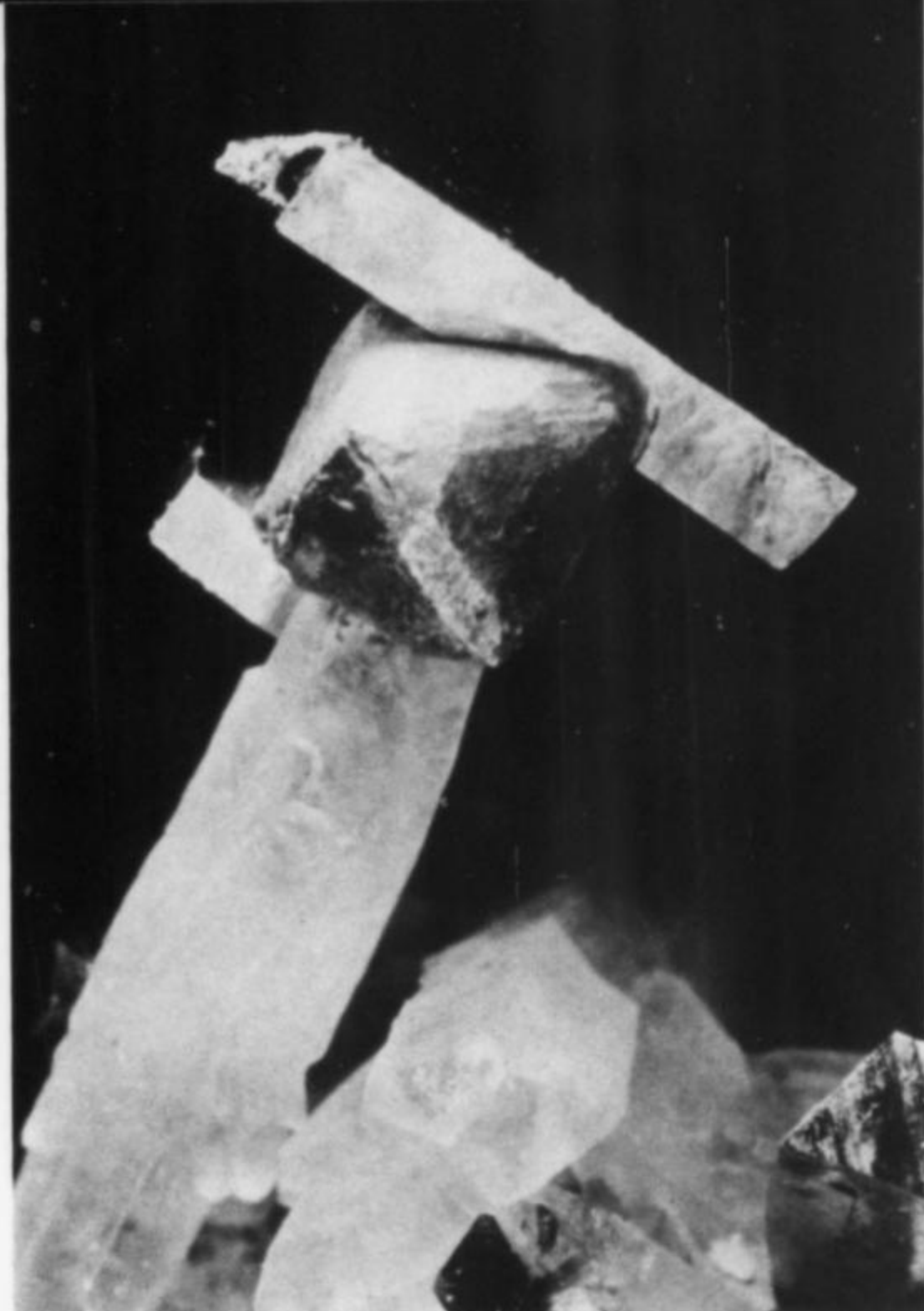
Fig. 8. Small elongated arsenopyrite crystal sitting on a small galena octahedron which is on quartz. The galena is about 3 mm.
