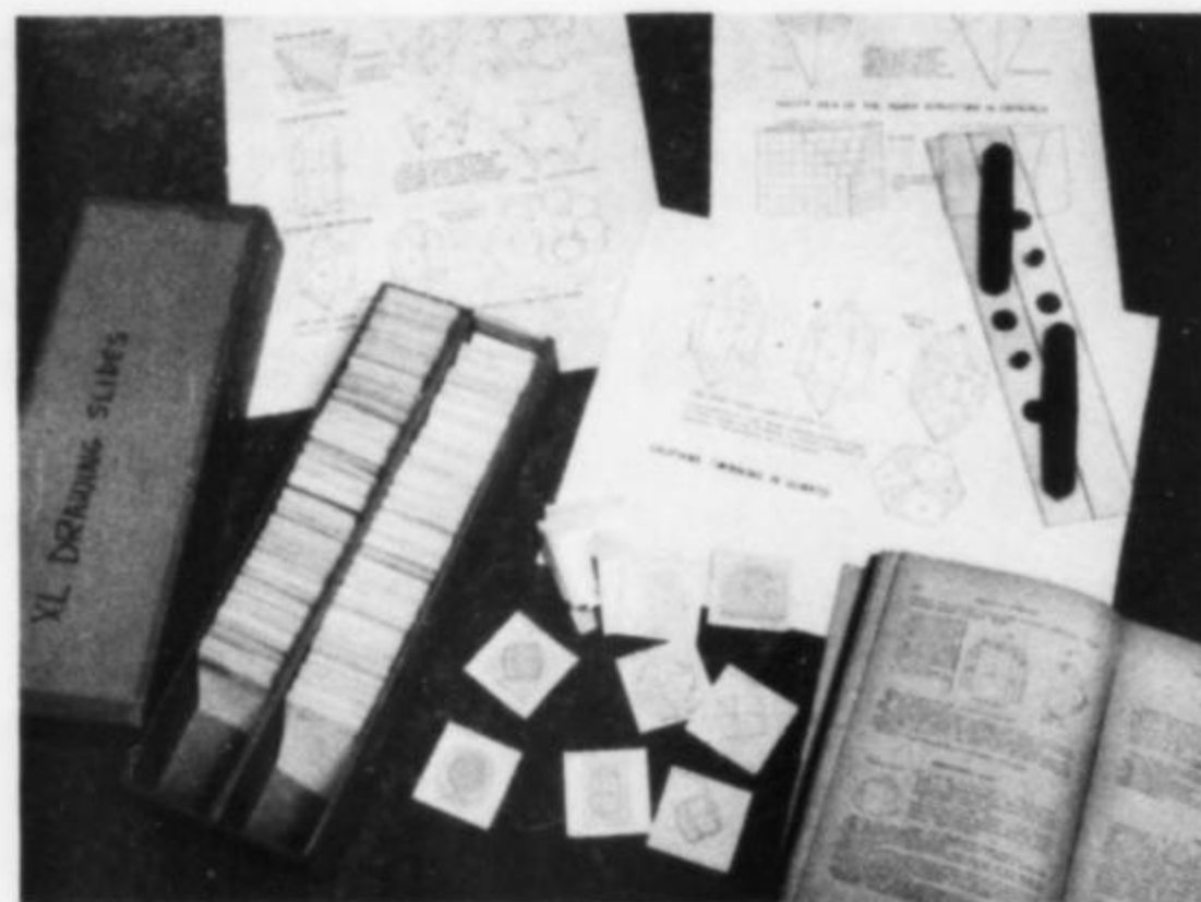
Dot projection slides and several drawings made by their use. Slides (2 x 2 in.) in storage box and in lower center.
