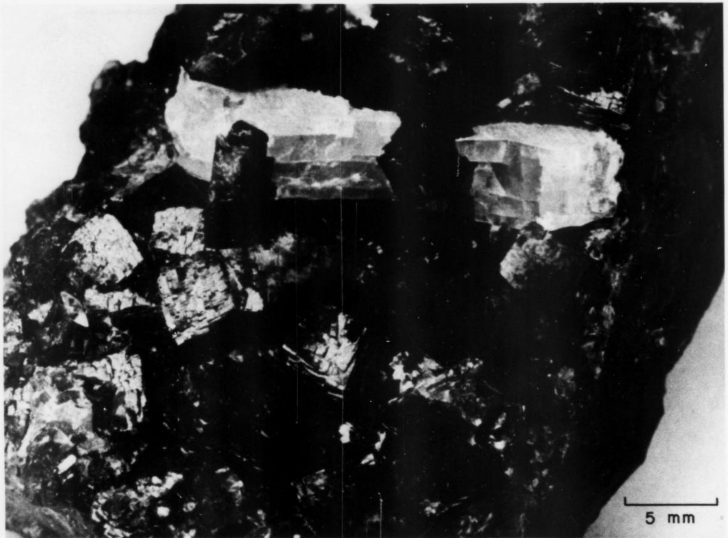
Fig. 1. Specimen of Iowa brown calcite with a crystal of white barite. Note dark color and curved nature of the crystals.
