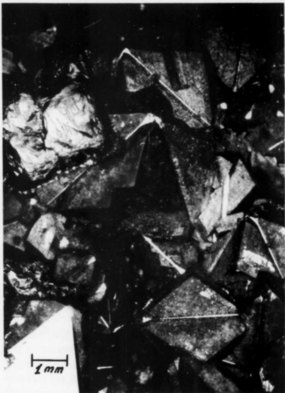
Fig. 1. Photomicrograph depicting general appearance of tennantite overgrowths on pyrite. Light lines traversing tennantite (gray) rhombuses are (011) of pyrite. Photograph by Julius Weber.
