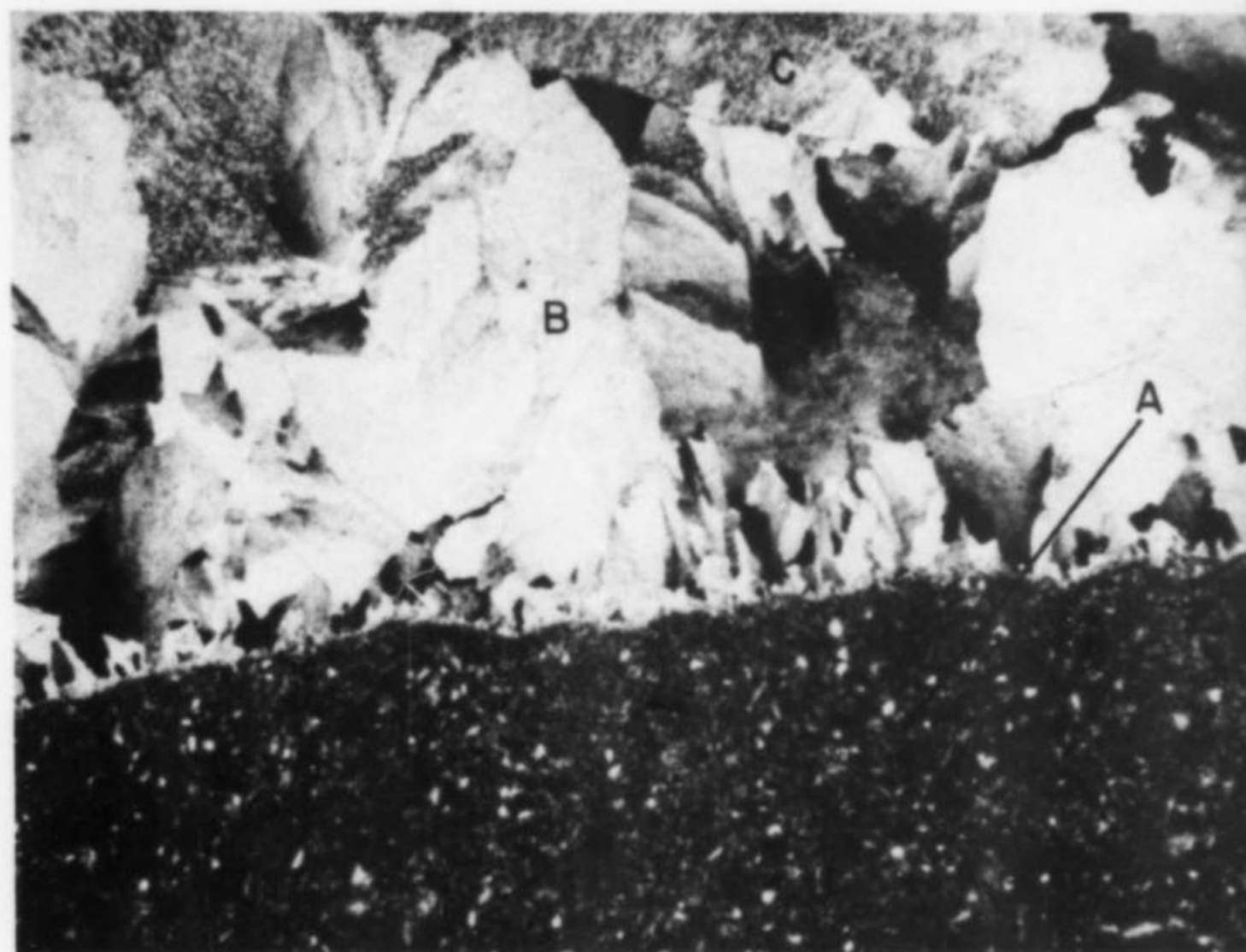
Fig. 2. Micrograph of Iowa brown calcite under crossed nicols at 35X. (a) black, siliceous, carbonaceous limestone, (b) brown calcite, (c) gray-translucent overgrowth of calcite with included sulfides.
