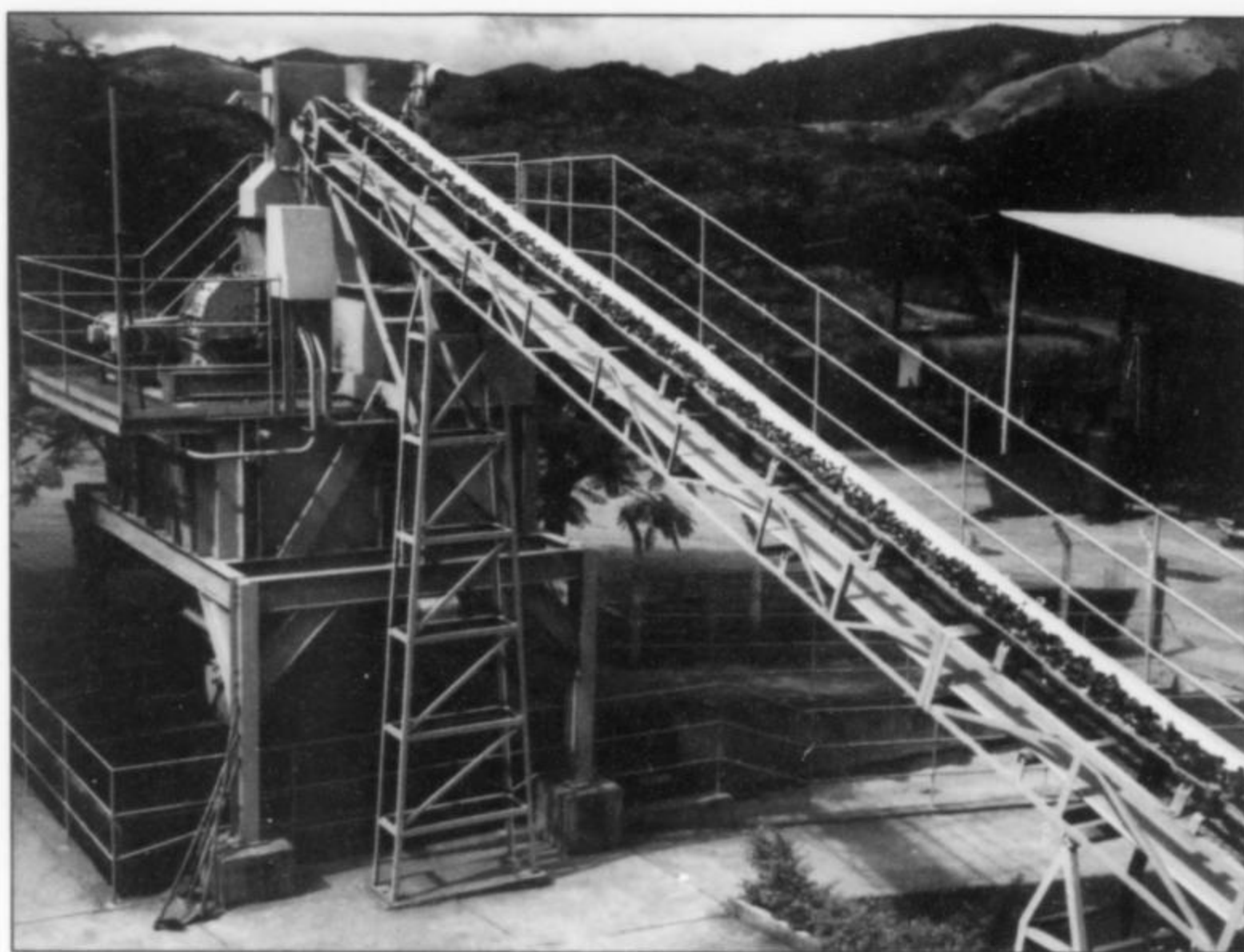
Figure 16. Overhead conveyor transporting coarse material for further sorting, Belmont emerald mine. Guido Steger photo, 2006.
