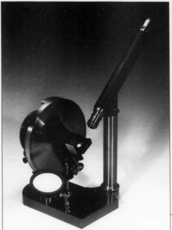
Figure 25. Wallerant-type total reflectometer with glass hemisphere. Please compare with Bertrand's hand held total reflectometer in figures 26 and 27. French, ca. 1890.
