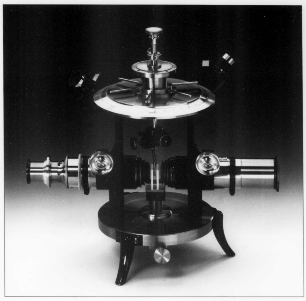
suspended goniometers, a direct-vision spectroscope could be fitted to employ the method of Soret (see later heading).
