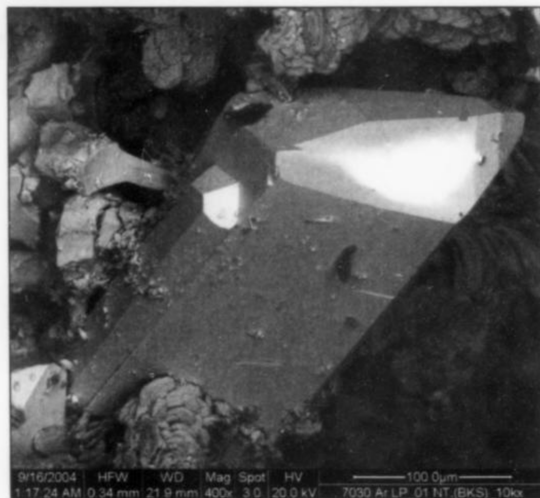
Figure 2. Scanning electron photomicrograph of stibioclaudeite, showing the terminal morphology of the crystals.
