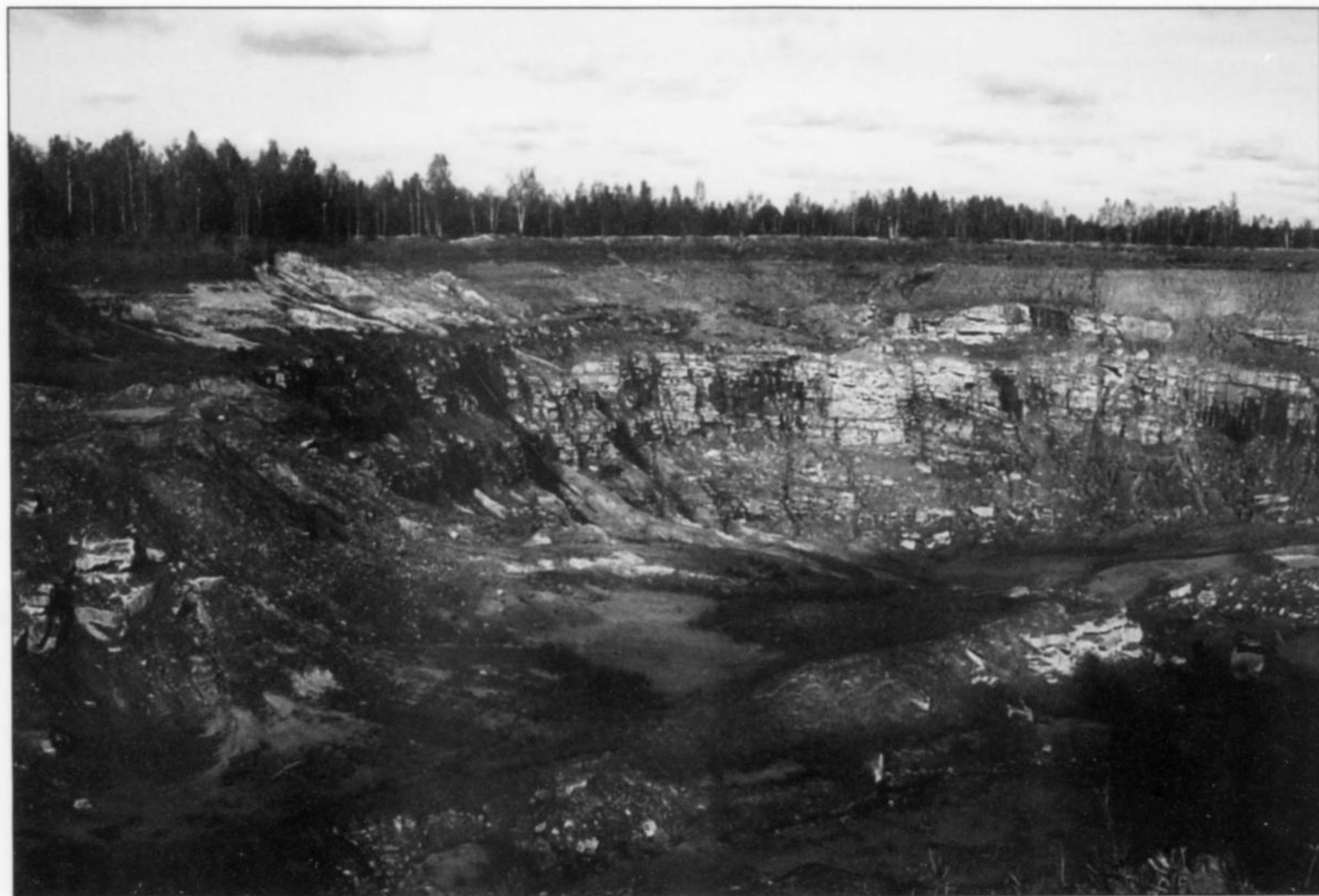
Figure 10. The Vishnyakovka open pit mined in the 1960s at Volodarsk-Volynski. Adits in the bottom of the pit (now buried) accessed 12 pegmatite chambers. Peter Lyckberg photo, 2007.
