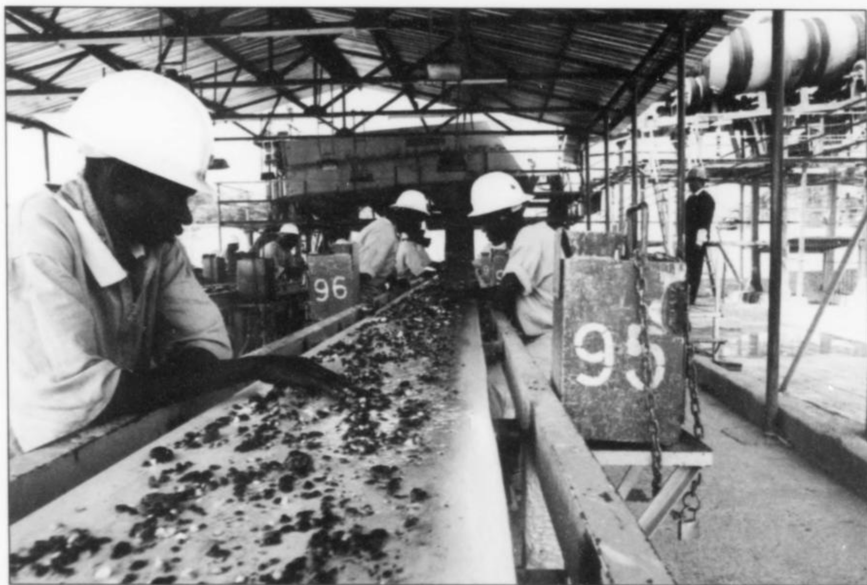
Figure 5. Sorting belt where emerald rough is hand-picked from crushed schist ore. Gemfields PLC photo.
