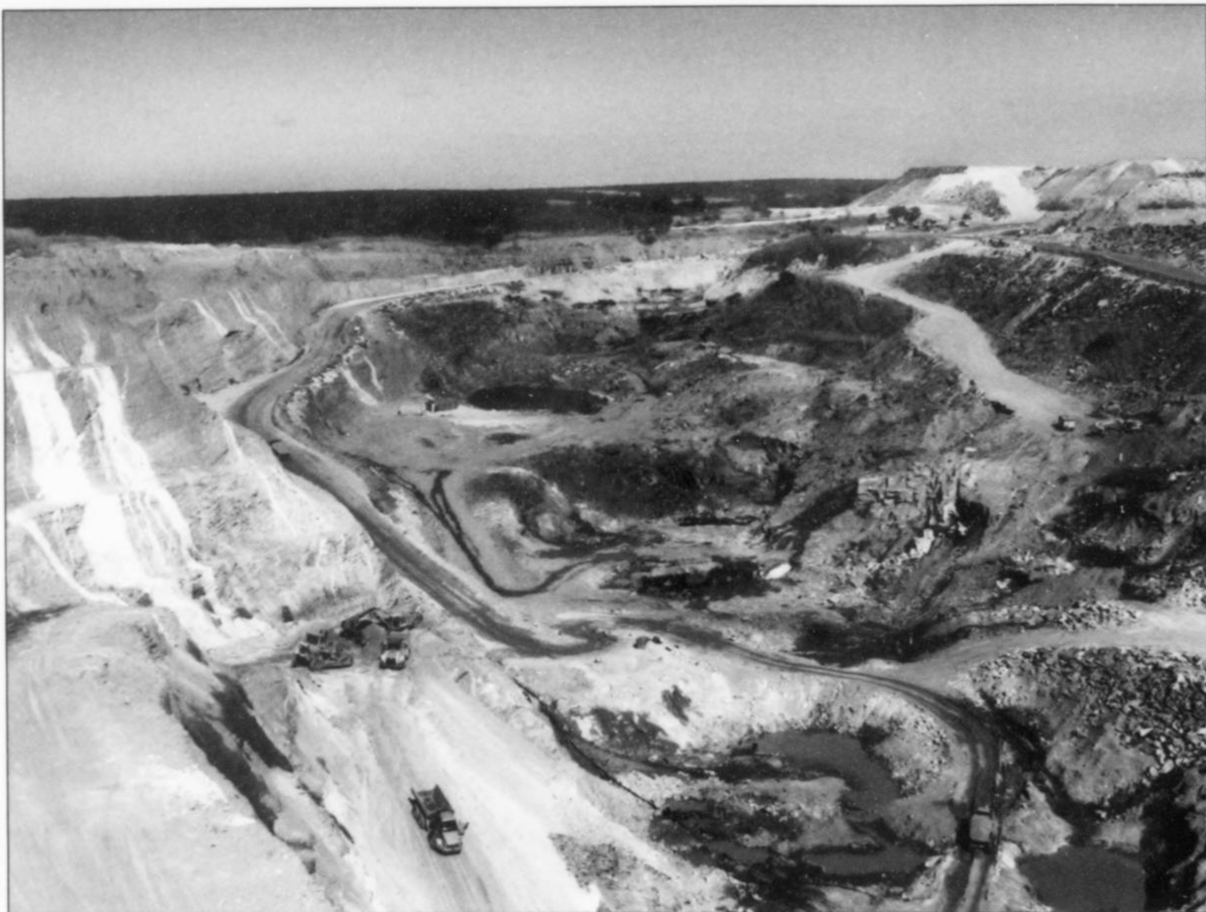
Figure 4. The open-pit Kagem mine (the merged Kagem Fwaya-Fwaya and Kagem Fwaya-Fwaya Extension F10 pits). Note the white pegmatite veins cutting across the country rock at left. Graham Sutton photo.
