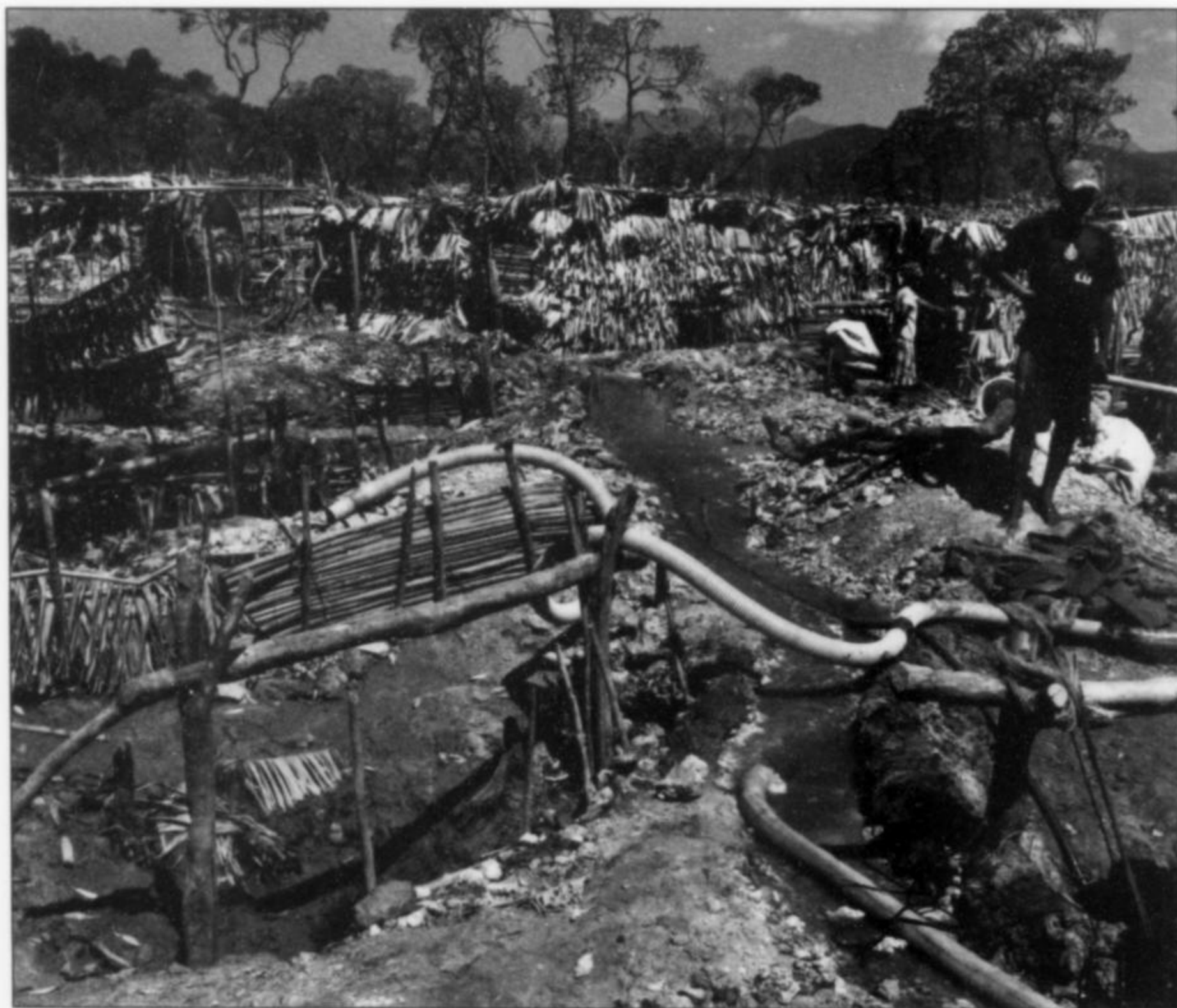
Figure 2. Drainage ditches, muck bunkers and pump hoses around pits in the mangrove swamp. Asia Gajowniczek photo.
