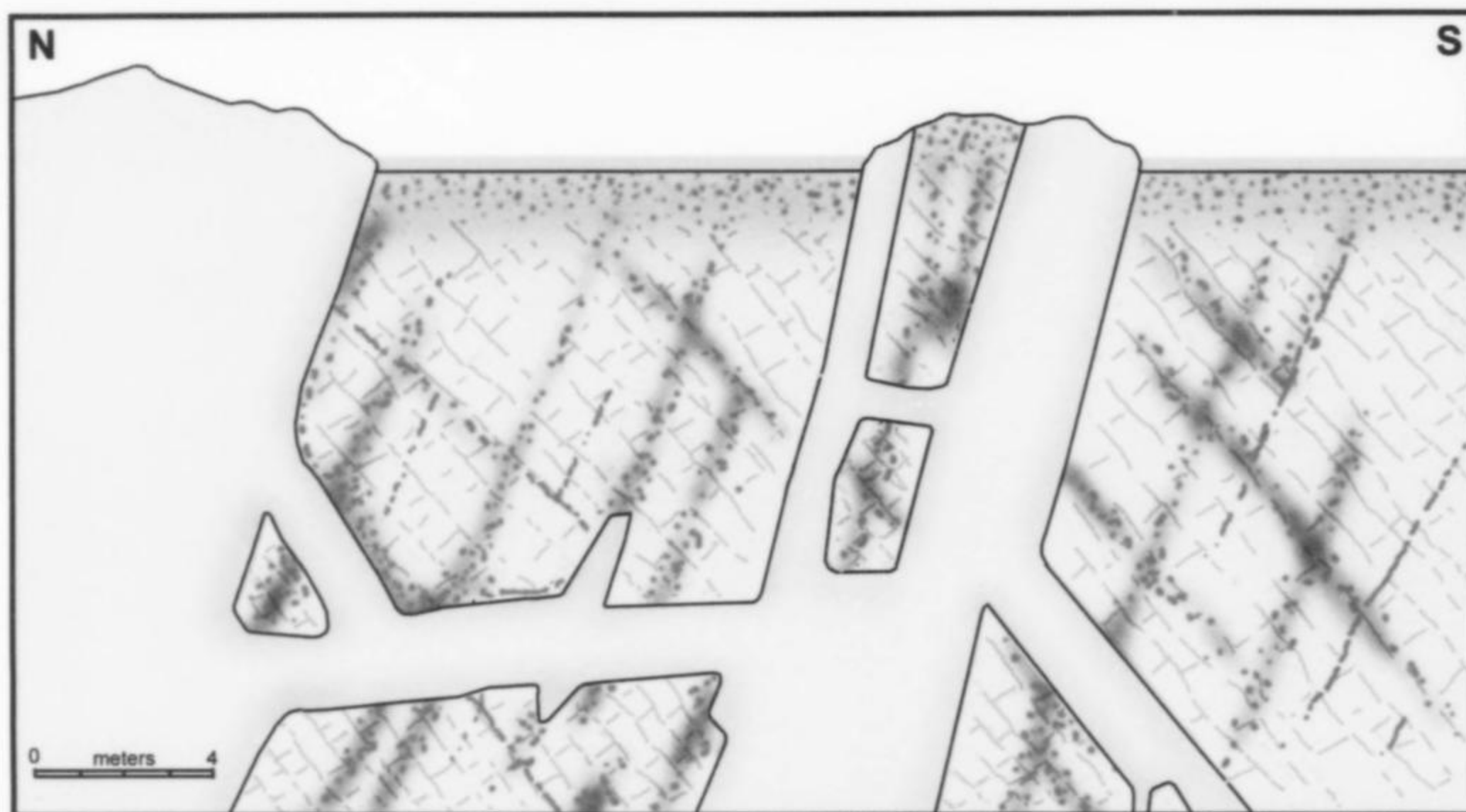
Figure 12. Interpretive geologic cross-section through the northern part of the demantoid deposit, showing high tide water (blue), near surface eluvial horizon of weathered rock containing broken and dispersed demantoid crystals (brown), interbedded sandstone and limestone dipping 40° to 60° south (tan) with zones that have been metasomatized (green), and demantoid-rich skarn veins (stippled green) developed along fractures, metasomatized areas and igneous contacts with the lamprophyre intrusion (pink).
