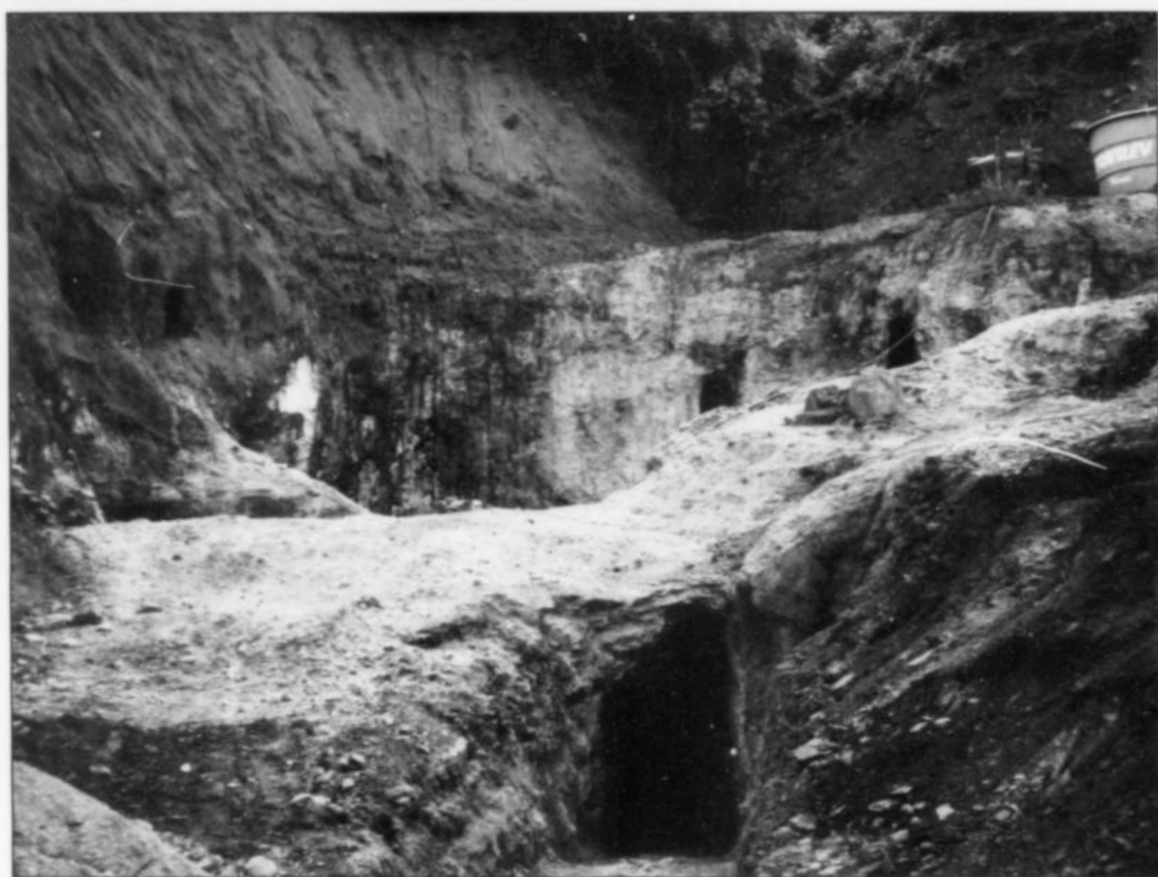
Figure 14. One of the many tunnel entrances in the laterite country rock of the Morro Redondo mine. Guido Steger photo.
