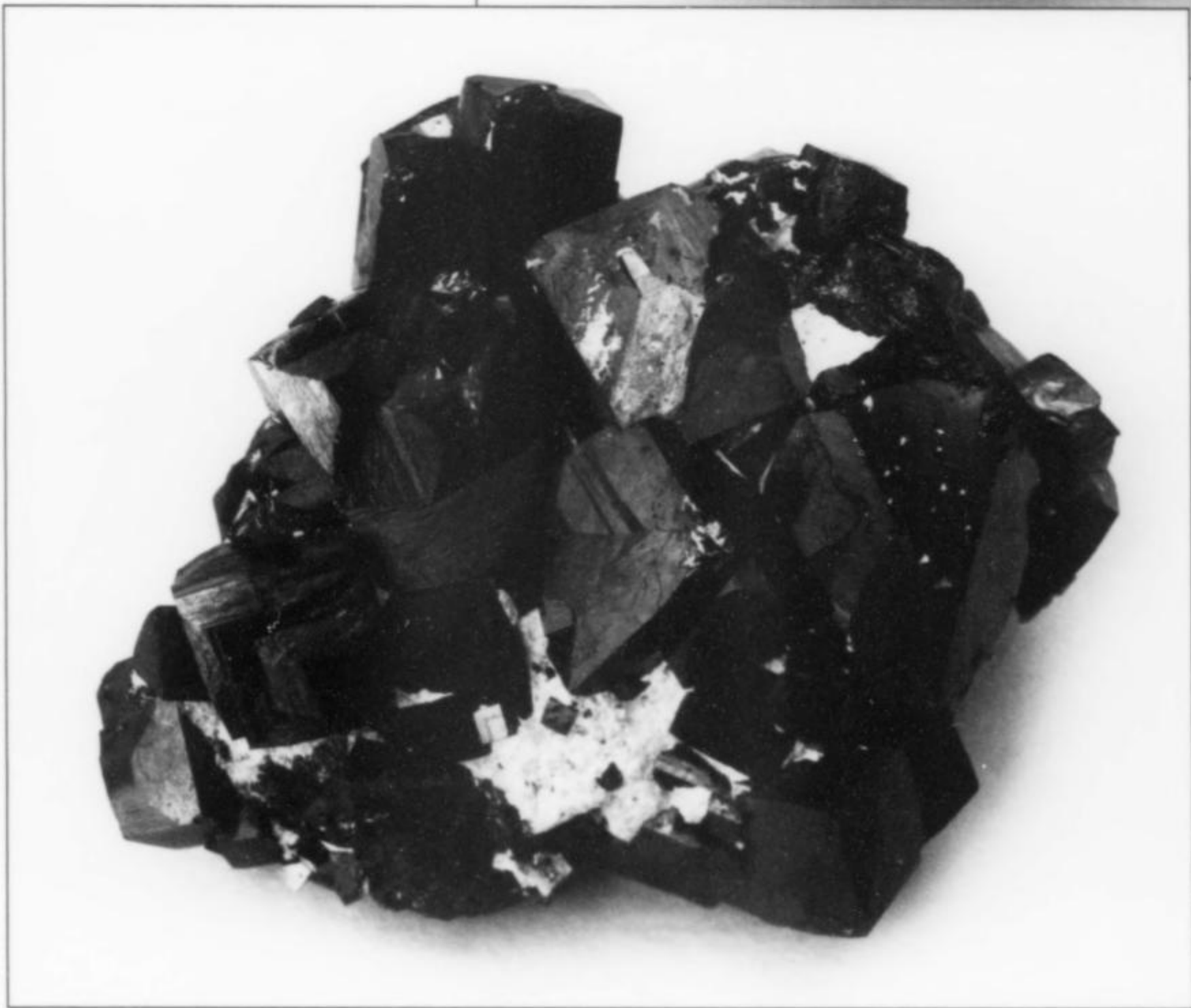
Figure 14. Tetrahedral magnetite crystals with minor cube faces and asymmetrical development of one of 8 octahedral faces, 9 cm wide. The specimen was embedded in halite/talc. Steve Chamberlain photo.
