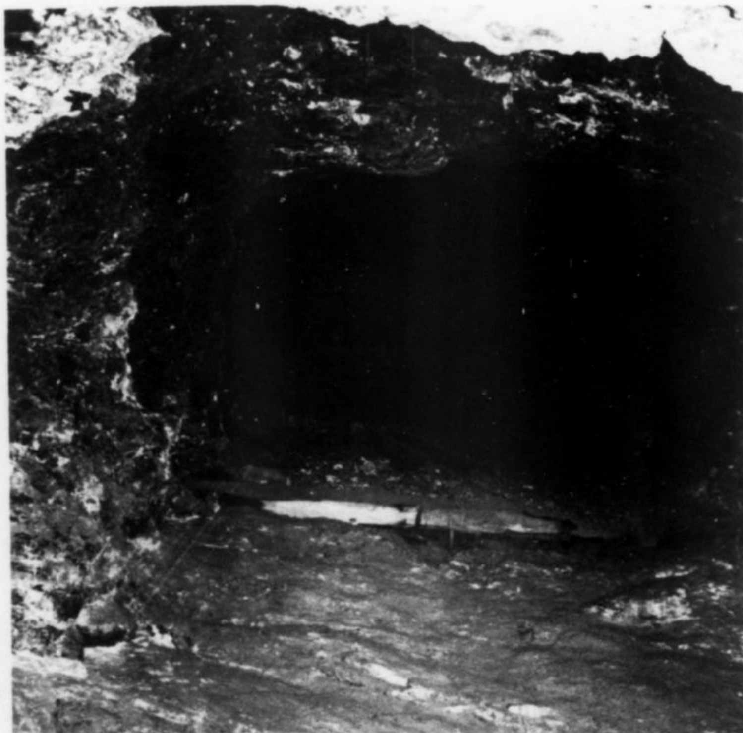
Fig. 9. A burned out incline in the Rowley mine, Maricopa Co., Arizona. Notice the charred remnants of shoring on the floor of the incline.
