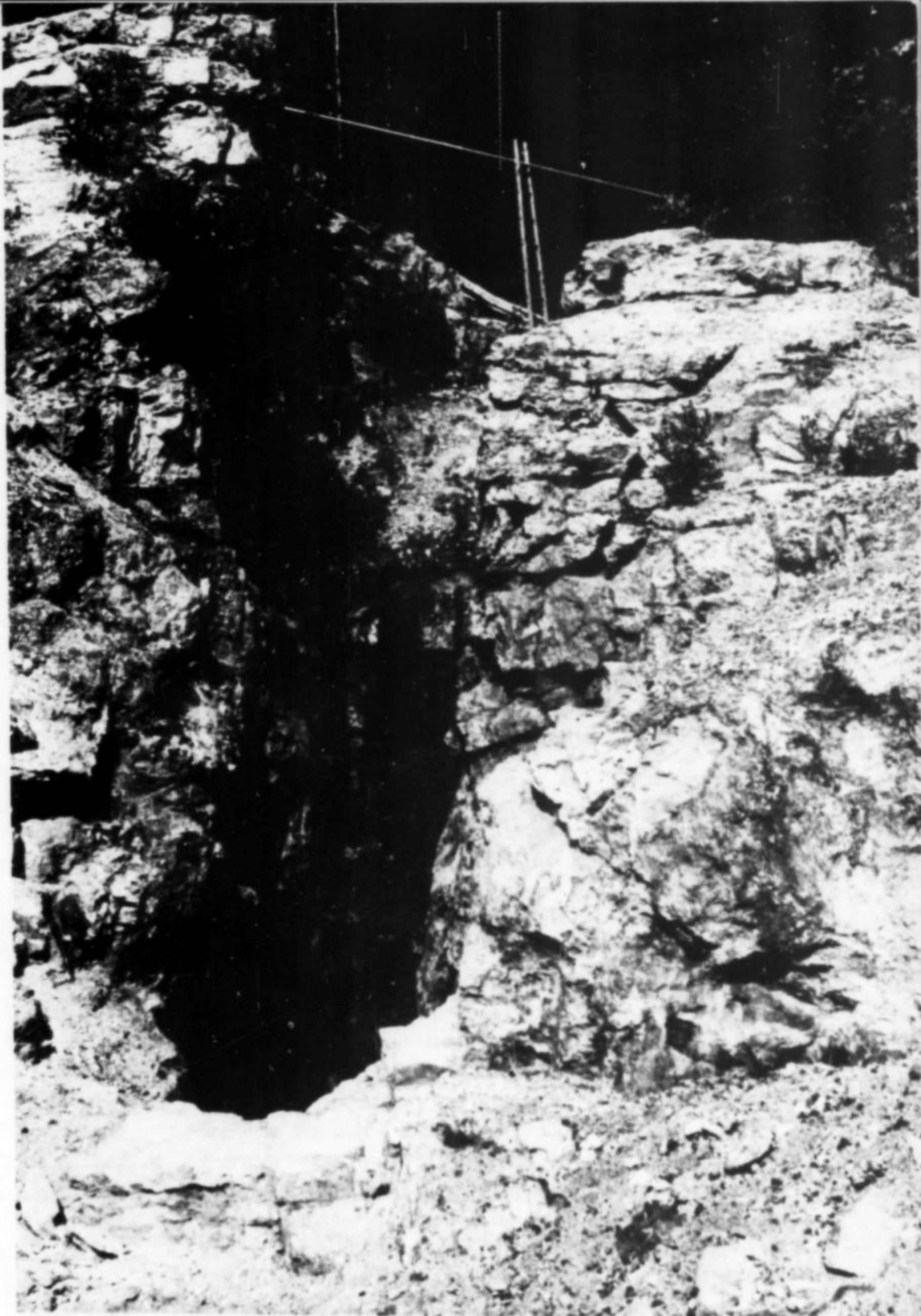
Fig. 3. Vertical shaft in the western part of the Palermo mine. Quartz core zone (white) and triphylite pods (gray) are visible in foreground.
