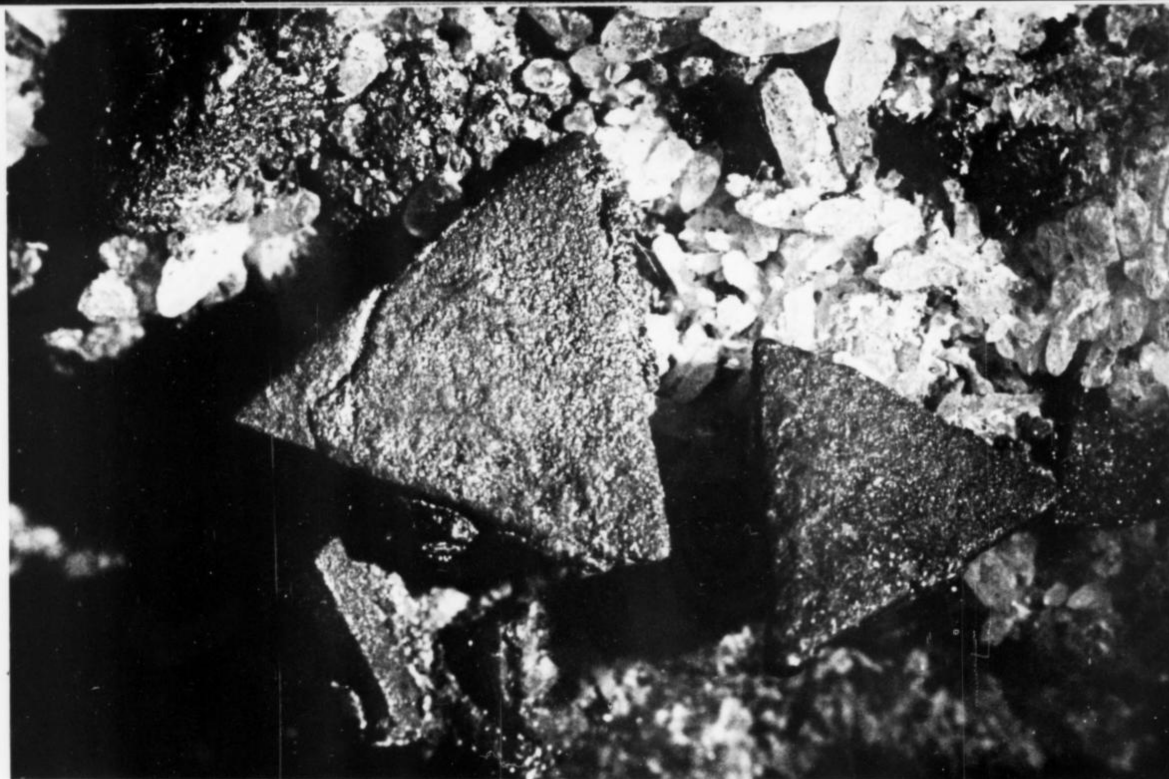
Fig. 1. Chalcopyrite, partially overgrown by pyrite, on quartz. The large crystal is 1 cm. Champion vein, 5 level, Tui mine.
