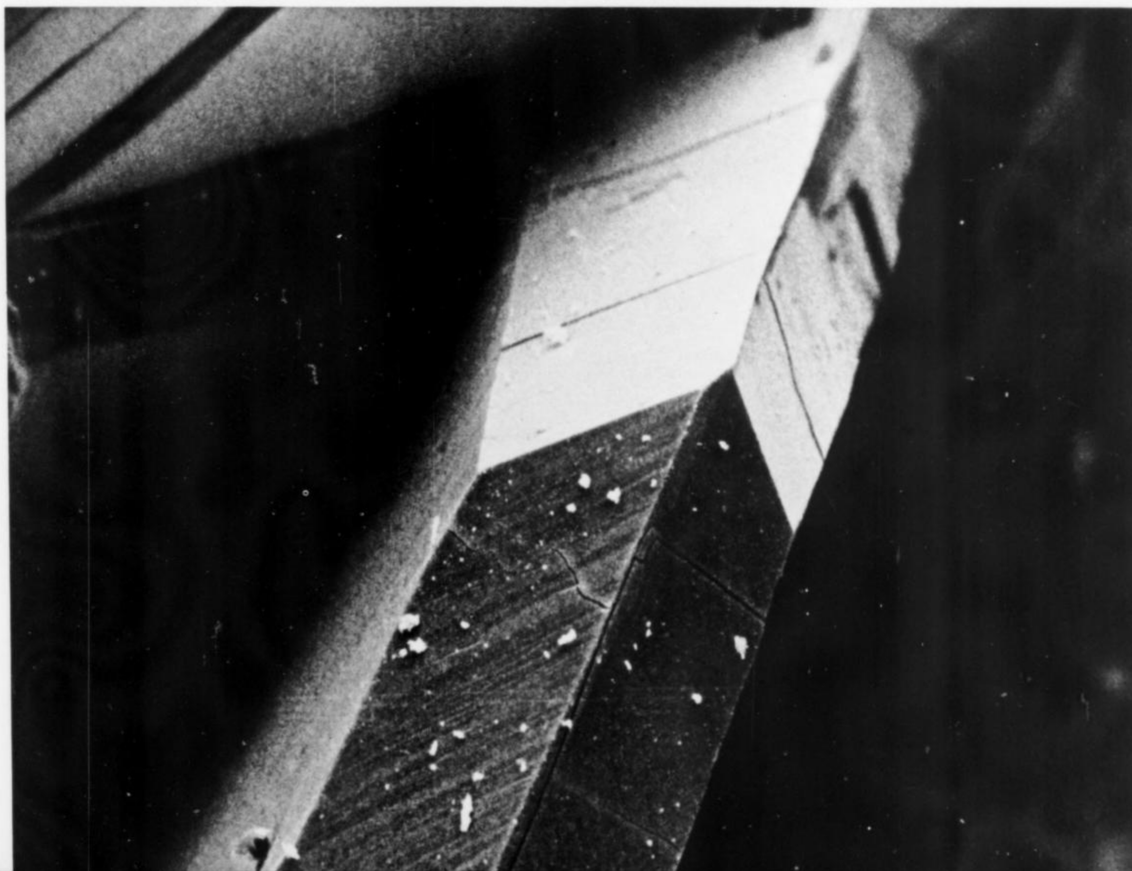
Figure 1. Complete crystal showing that the offretite layer extends over all of the crystal faces. 220X.
