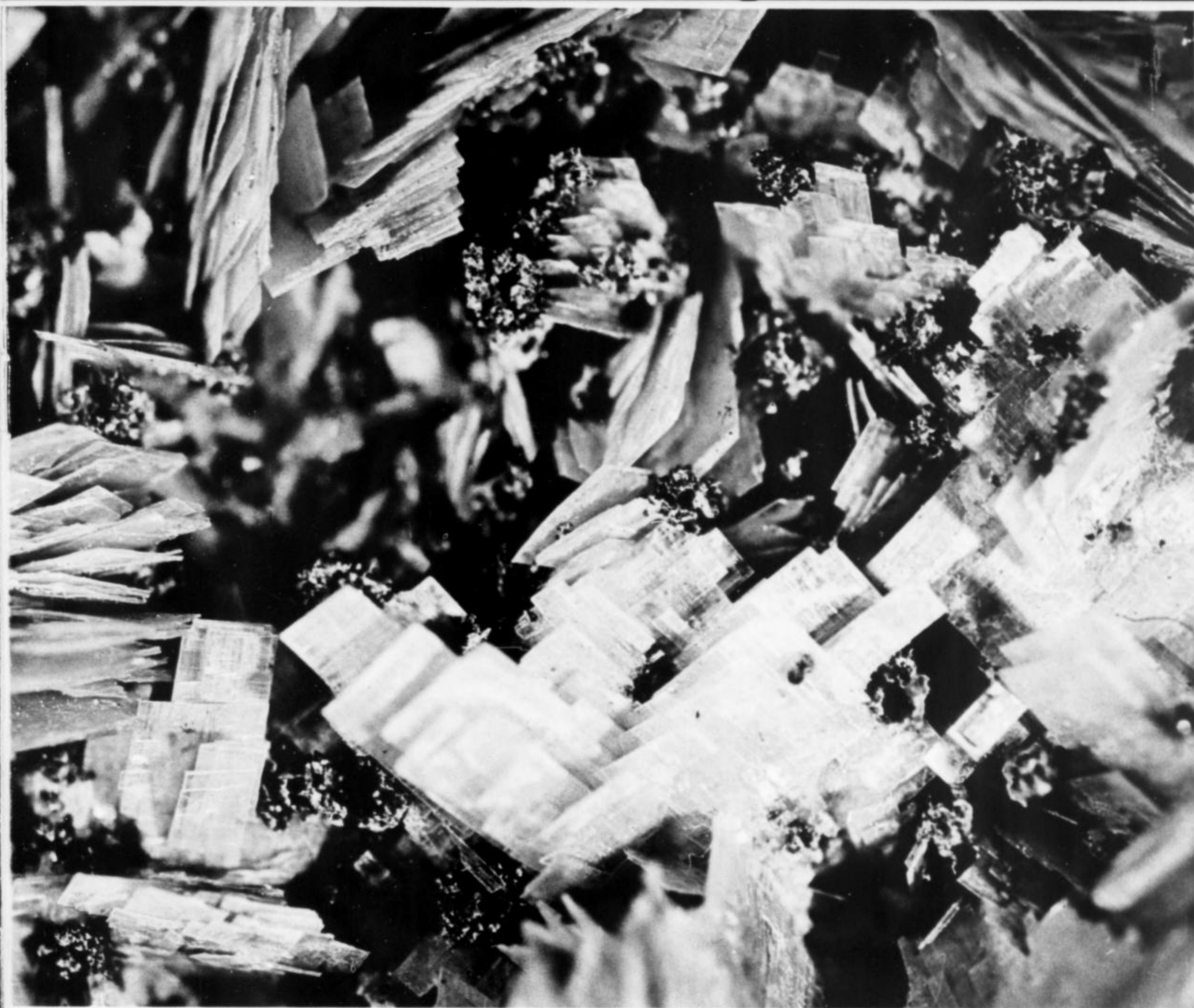
Figure 19. Aggregates of meta-uranocircite crystals on pelitic matrix; mammillary uraninite is usually found, with renardite, in association with these crystals.
