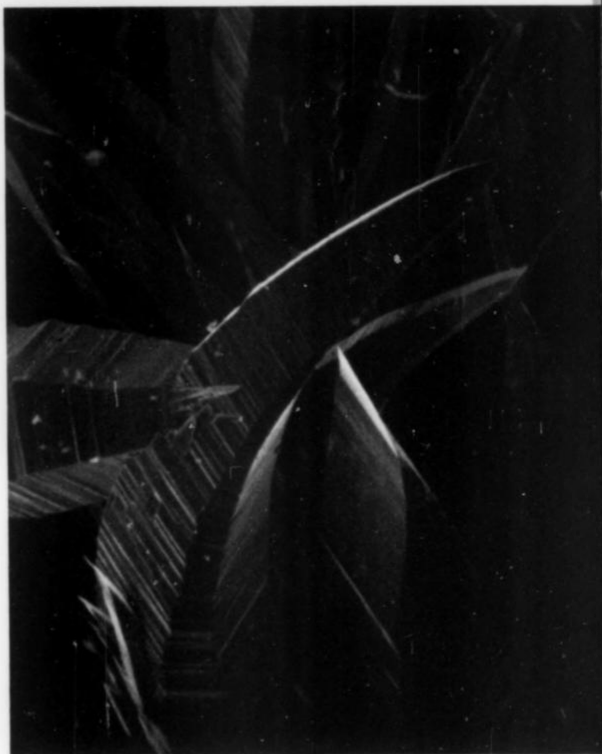
Figure 2b. Strontianite crystals at a greater magnification showing striations due to alternation of \{010\}/\{0kl\} and \{110\}/\{hhl\} forms.
