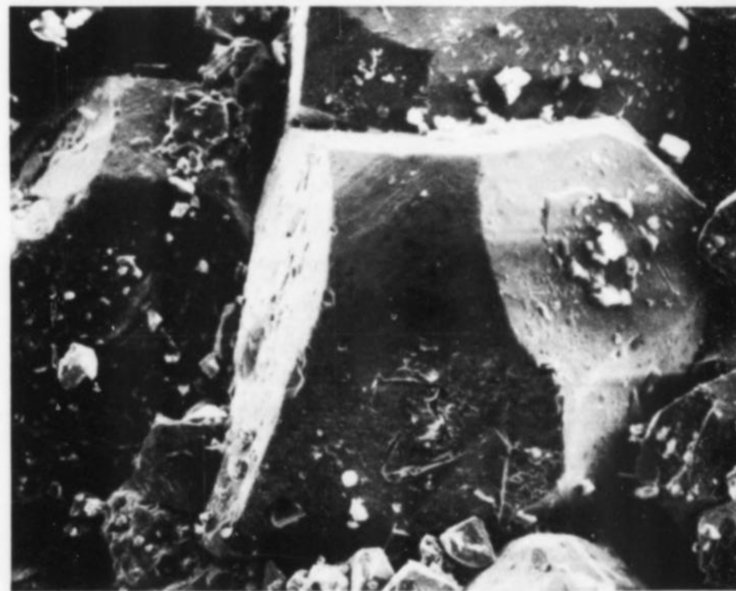
Fig. 2. (above) and (below). Scanning electron micrographs of pyrite crystals in the center of the concretions. Magnification: a, 100 x; b, 150 x.
