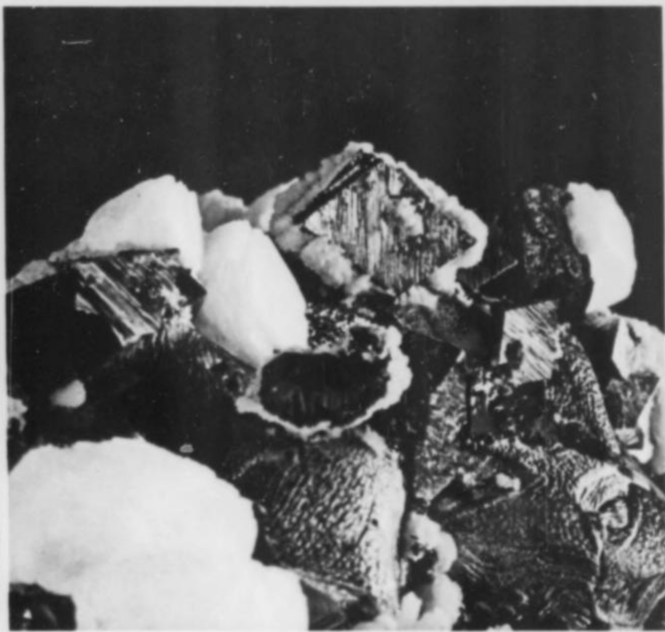
Figure 5. Arsenopyrite rimmed with calcite on galena (specimen no. 31216). Width of larger arsenopyrite is 1 cm.
