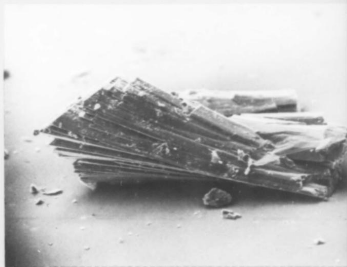
Figure 3. Keyite: a typical sub-parallel group of crystals. The apparent size of \{011\}:(011) is increased by divergence. SEM, 500x
