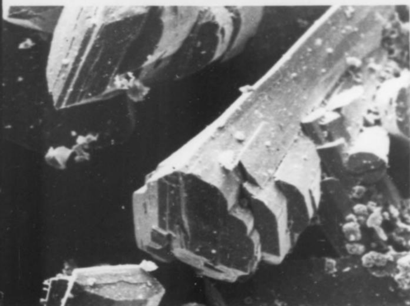
Figure 2. Keyite crystals showing forms h\{210\} , m\{110\} , b\{010\} , and q\{011\} ; the largest crystal shows the terminal form \{201\} (?). SEM, 500x.
