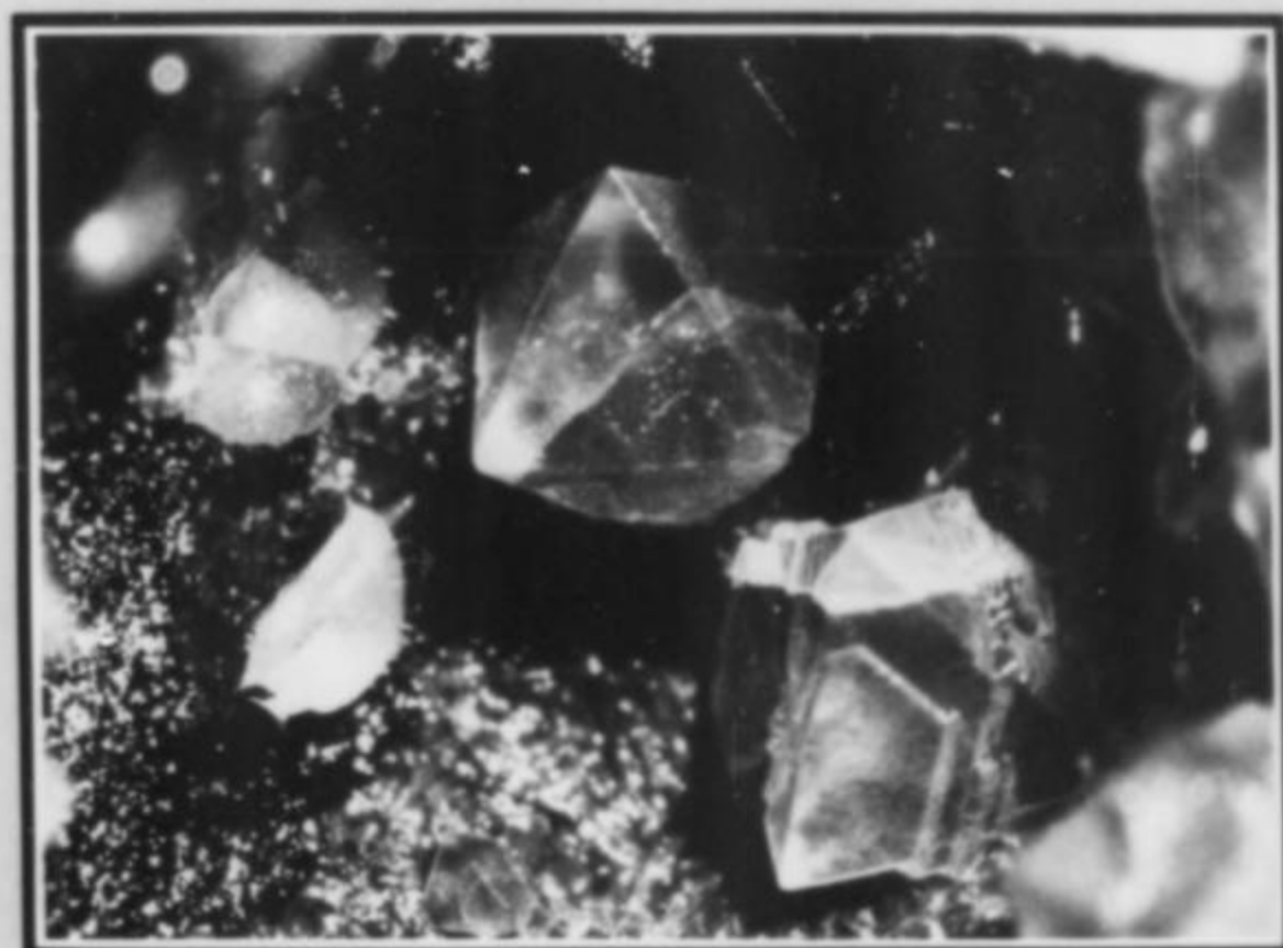
Figure 4. (below) Faujasite octahedrons (0.5 mm) with phillipsite spherules and erionite-offretite needles from Limberg near Sasbach, Kaiserstuhl, Baden. Limberg is the type locality for faujasite, first described by Damour in 1842. The mineral was found in crystals up to 3 mm (Wimmenaur, 1959) but the more common size of 0.5 mm crystals can still be collected; the pictured specimen was collected in March of 1976. Faujasite with phillipsite and erionite-offretite has been described by Rinaldi (1976) and Hentschel (1976). (Collection of V. Betz)
