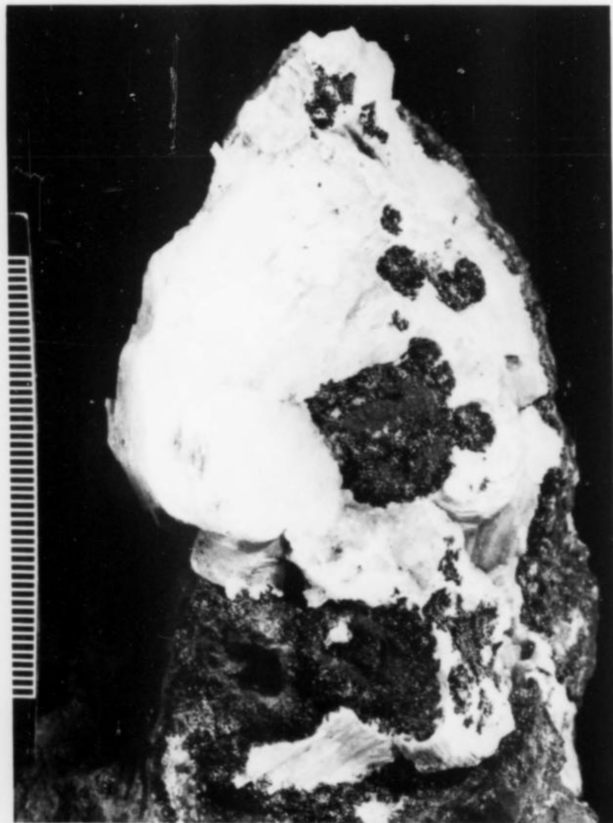
Figure 4. Cleaved hydrocerussite crystal (pearly white) associated with a manganese oxide matrix (black), from the Merehead quarry. Maximum diameter = 6.5 cm (B.M.No. 1969, 162)
