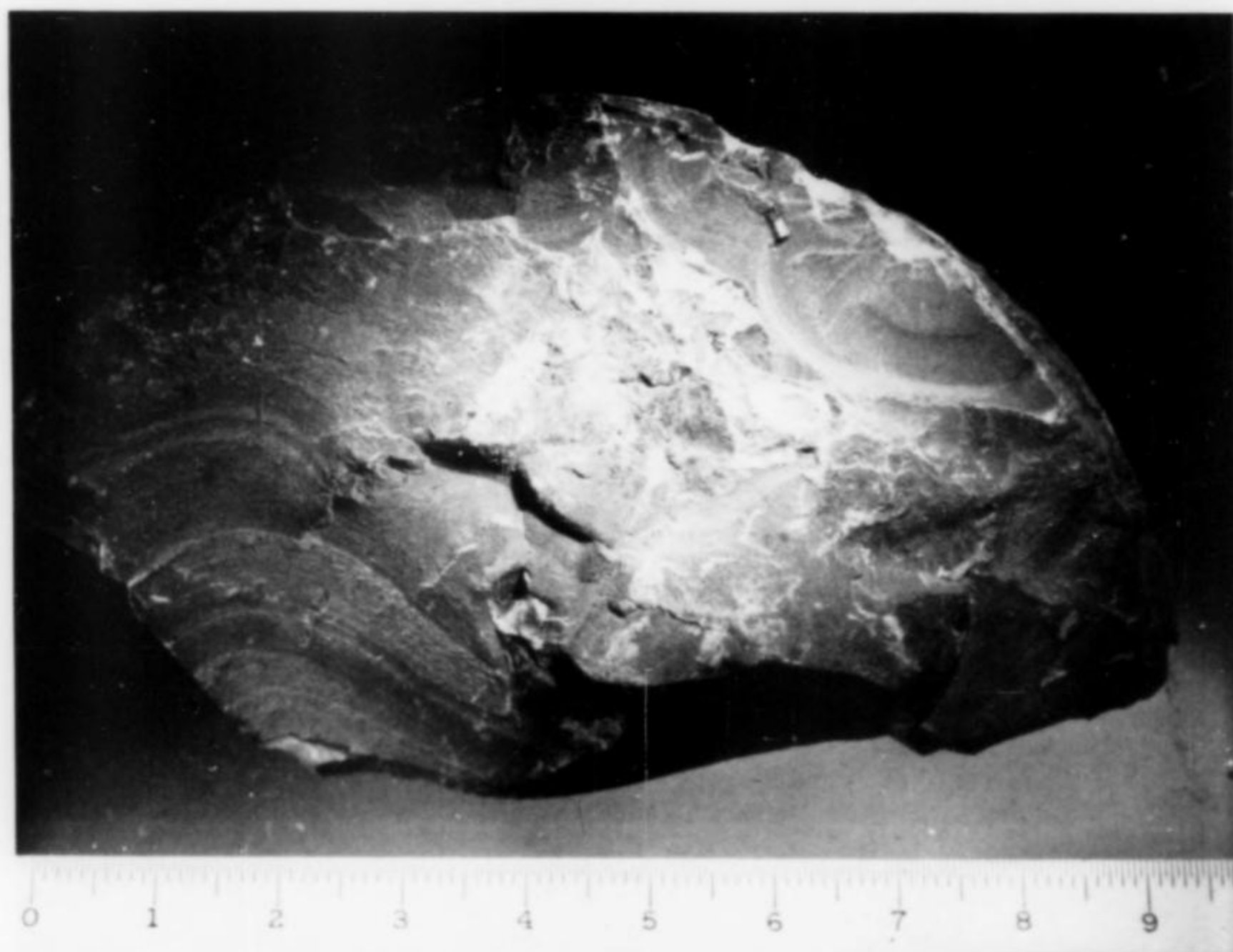
Figure 3. A few years later a core sample from another well drilled in the area showed a tiny crystal (edge of core, above figure 6 on centimetre scale) referred by Allan P. Bennison, geologist to the U.S. Geological Survey, for identification. It was found to be a complex titano-boro-silicate, leucosphenite, an extremely rare mineral previously known only from alkalic pegmatites. Naturally, it was at first thought to be likewise of igneous origin, a detrital mineral washed into the Green River Lake in the Uinta Basin of Utah.
