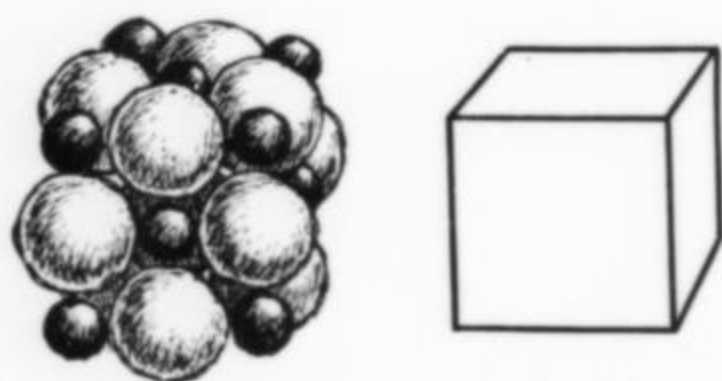
Figure 4. Arrangement of sodium and chlorine ions in halite. The large circles represent chlorine and the small black circles represent sodium.
