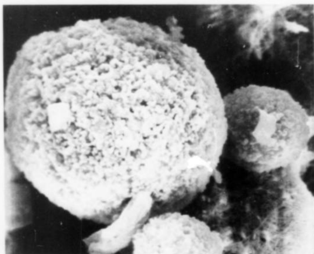
Figure 10. A scanning electron micrograph of pyrolusite on calcite. The spherical pyrolusite mass is about 0.02 mm in diameter.
