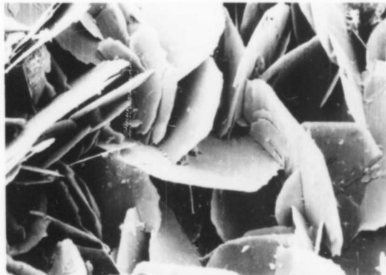
Figure 4. Micrograph of red, earthy hematite. Individual plate-like crystals average about 0.15 mm across.
