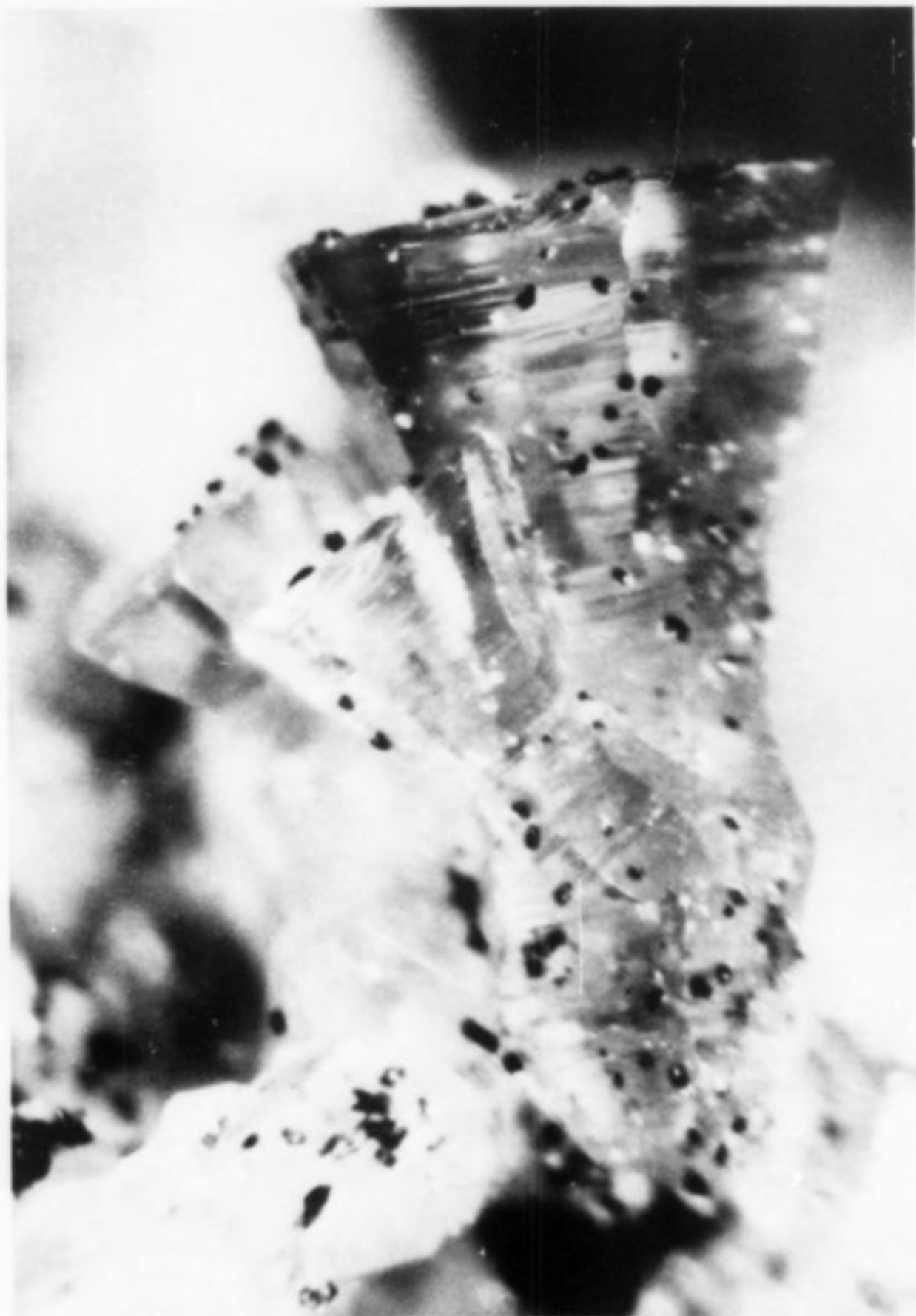
Figure 1. Weloganite crystals (grayish yellow at the base, amber at the top; height of largest crystal: 2mm) from the Francon quarry, Montreal Island, Quebec. Les Horvath collection.
