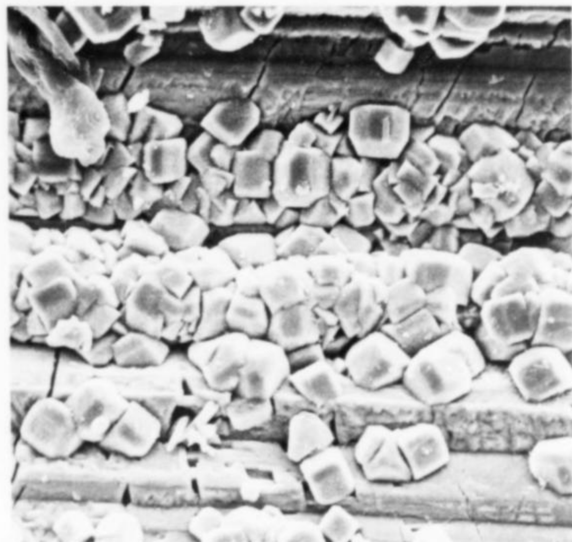
Figure 1. Isometric vaesite crystals on a striated polydymite crystal from the Sweetwater mine, Reynolds County, Missouri. (860 X)
