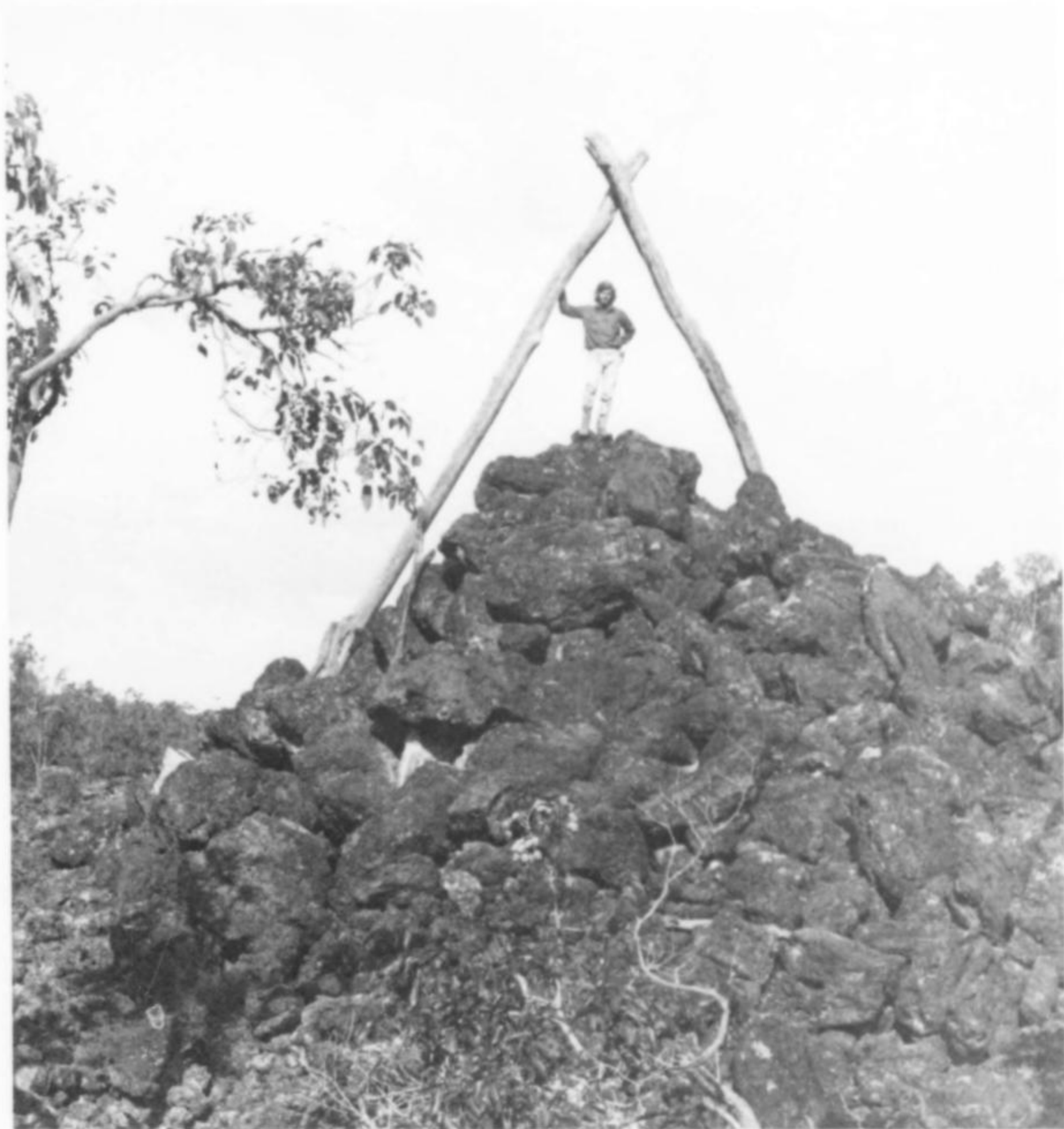
Figure 1. Laterite waste piles, these are the work of early tin miners who washed and dug alluvial material from beneath an extensive laterite capping. When the capping collapsed the blocks were hoisted from the pit and placed in waste heaps.
