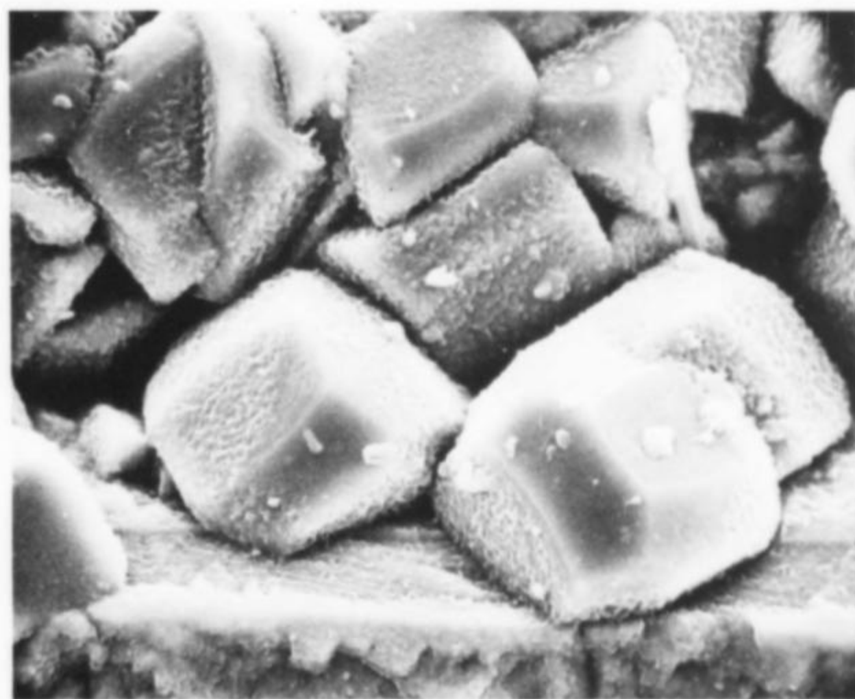
Figure 2. Vaesite crystals on polydymite from the Sweetwater mine, Reynolds County, Missouri. (2900 X)
