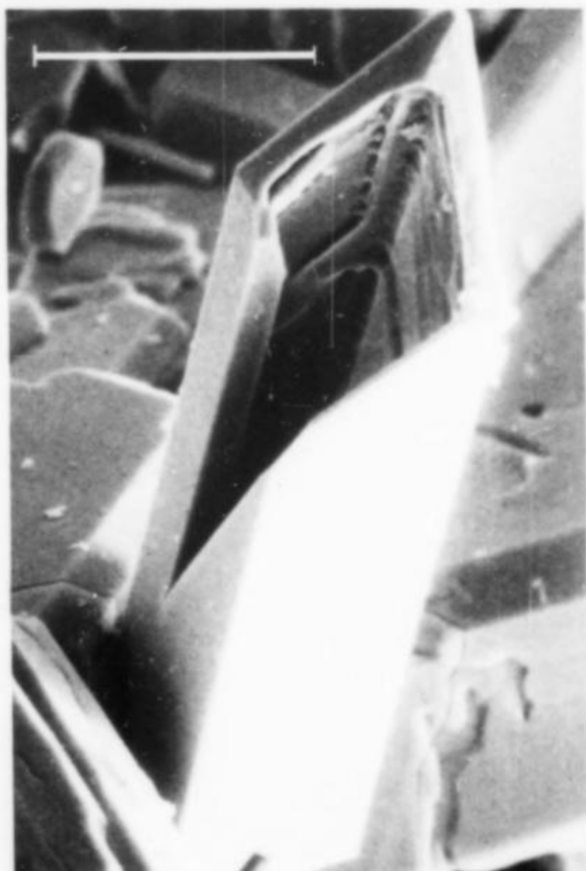
Figure 3. A cavernous zircon crystal with incomplete development of both the pyramid and prism faces. Note the ribbed appearance of the internal cavity.
