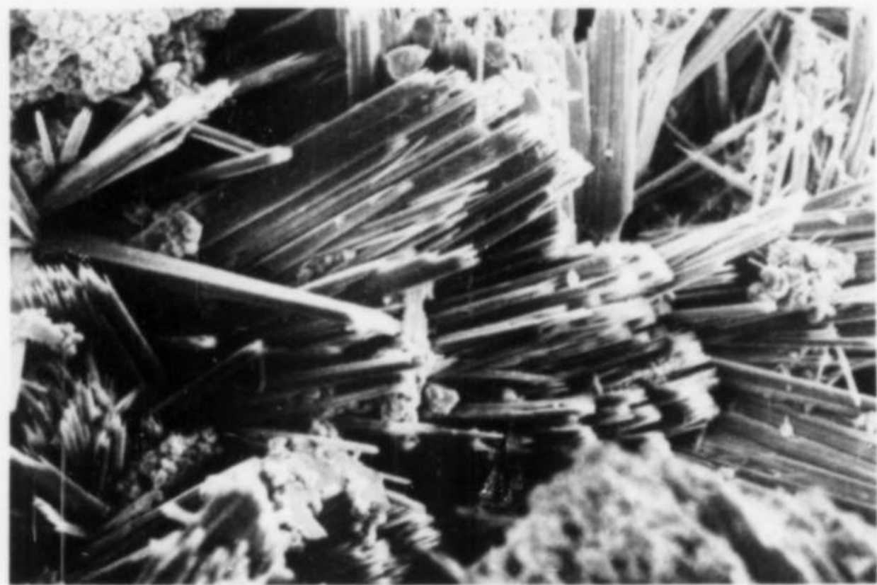
Figure 9. Acicular crystals of dark green rockbridgeite up to 0.1 mm in length (SEM photo) from near Jacksonville, Alabama.
