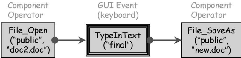
FIG. 21. A plan consisting of component operators and a GUI event.
