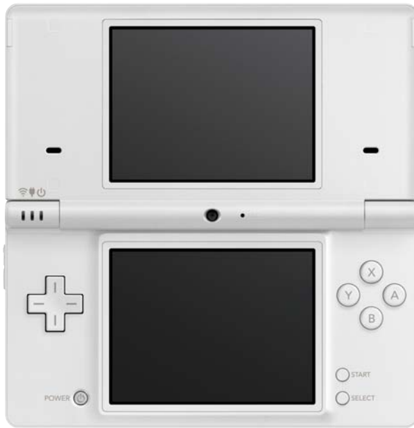
FIG. 5. The Nintendo DS mobile gaming console offers one standard screen and one touch-sensitive screen. Its updated version DSi—which is depicted here—also contains two cameras, one of which faces the user. Image © 2008 Nintendo of Europe GmbH. Used with permission.
