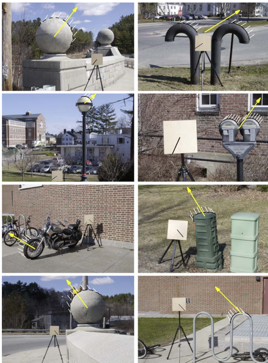
FIG. 2. Shown are eight images with the extracted occluding boundaries (black), individual light source estimates (white), and the final average light source direction (large arrow). In each image, the cast shadow on the calibration target indicates the direction to the illuminating sun, and has been darkened to enhance visibility.
