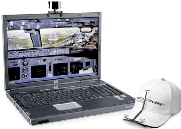
FIG. 6. TrackIR 4 employs reflectors affixed to a cap or LEDs attached to a headset to determine the position and orientation of the user's head. Image © 2008 NaturalPoint. Used with permission.
