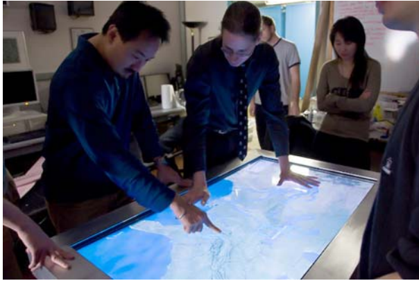
FIG. 2. TacTile: a 52-in. high-definition LCD-based multitouch table.
