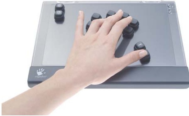
FIG. 3. The Ergodex DX1 system allows placing keys anywhere on its surface. Image © 2008 Ergodex. Used with permission.
