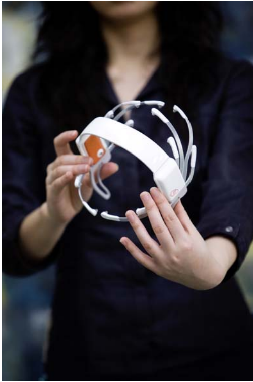
FIG. 10. The Emotiv EPOC hardly resembles the bulky EEG caps used in traditional systems. Image © 2008 Emotiv Systems. Used with permission.
