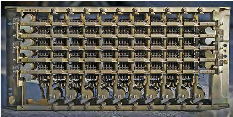
FIG. 10. Crossbar switch manufactured by Western Electric (1970).
