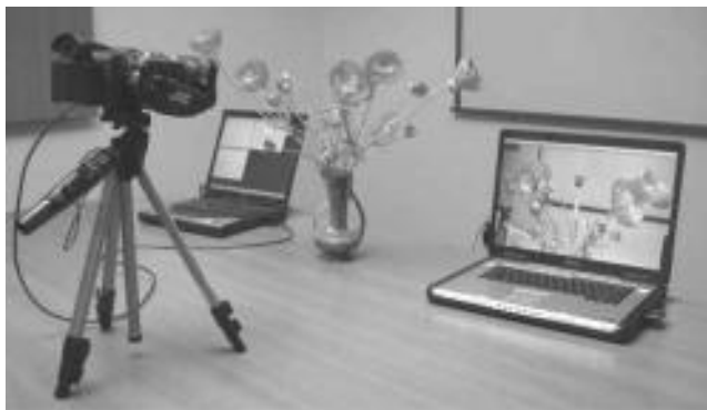
Figure 1.10 HD transmission over a wireless, ad hoc link (802.11a) between two laptops in the laboratory.
