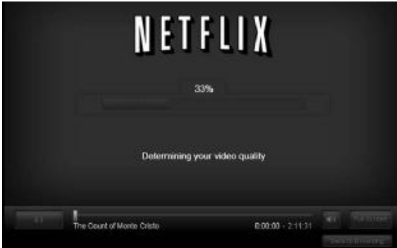
Figure 3.1 Netflix software judges the level of quality allowed for by your bandwidth and then streams out the video.
