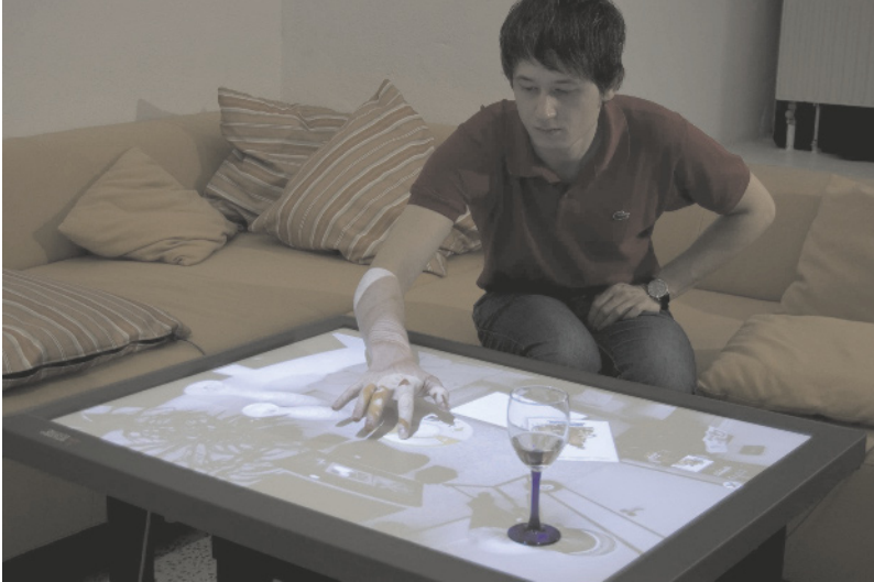
The DiamondTouch Table. Based on an array of antennas embedded in the touch surface, the DiamondTouch can detect up to four different users simultaneously.
