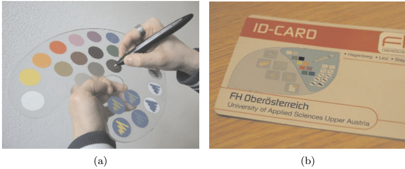
FIGURE 16 Different possibilities for the additional interaction. We either support a unique palette (a) or special ID cards where the additional functions are printed on the backside of each card (b).
