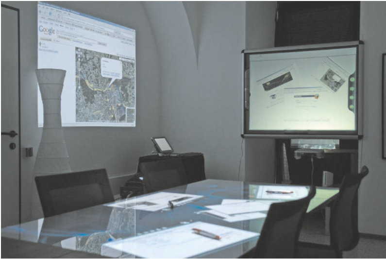
FIGURE 6 The interactive room consisting of a digital tabletop, a digital whiteboard and a presentation display.
