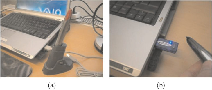
Anoto pens are available in two versions: a USB only version (a) and a Bluetooth streaming version (b).
