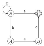
Note that d is a partial function: for example d B a is not defined. We can make d into a total function by introducing a new 'sink' state, the result state of all undefined transitions. For example, in the above automaton we can introduce a sink state D with d D x = D for all terminals x, and d E x = D for all states E and terminals x for which d E x is undefined. The sink state and the transitions from/to it are almost always omitted.
