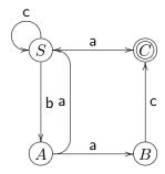
The nondeterminicity of this automaton appears in state A: two outgoing arcs of A are labelled with an a. Suppose we add a new state D, with an arc from A to D labelled a, and we remove the arcs labelled a from A to B and from A to B. Since D is a merge of the states B and B we have to merge the outgoing arcs
