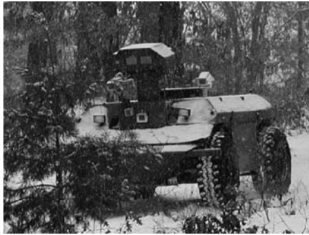
Figure 12.17: The Automated Cross-Country Unmanned Vehicle (XUV) is equipped with laser radar and other sensors, and uses Stentz’s algorithm to navigate (courtesy of General Dynamics Robotic Systems).
