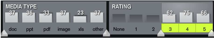
Fig. 4.5C The ContentLandscape application (see Sect. 4.5.3) combines bar chart representations with slider controls for range selection
