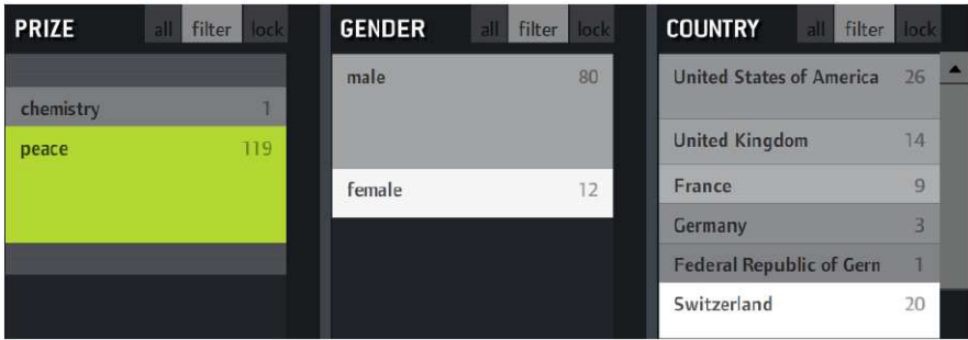
Fig. 4.16 Elastic lists indicate the number of matched resources in scaling list entry height. Additionally, unusually high proportions (compared to the global distribution) are indicated by brightness of the list entries
