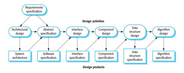
Figure 4.7 A general model of the design process
