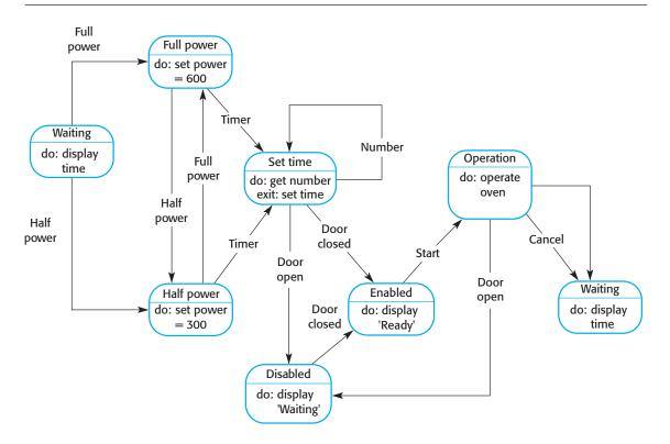
Figure 8.5 State machine model of a simple microwave oven alarm system discussed in Chapter 13 responds to stimuli from movement sensors, door opening sensors, and so on.
