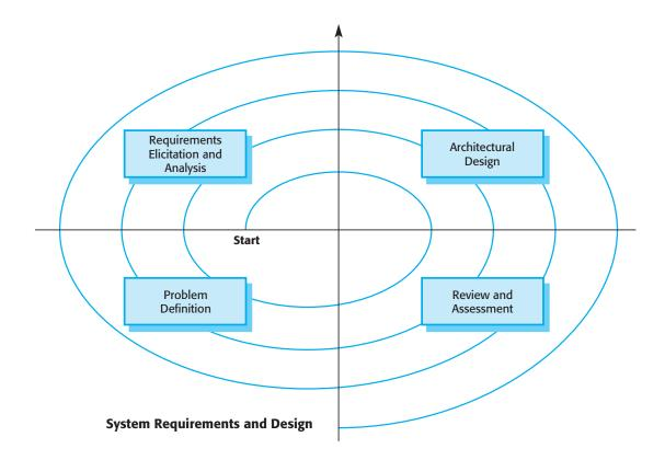
Figure 2.5 A spiral model of requirements and design or, if the sub-system is a software system, part of the requirements specification activity for that system. You should also try to identify relationships between sub-systems at this stage.
