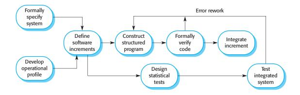
Figure 22.10 The Cleanroom development process refinement of the specification. A limited number of constructs are used and the aim is to systematically transform the specification to create the program code.
