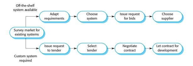
Figure 2.10 The system procurement process
