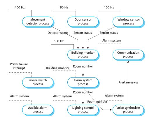
Figure 15.8 Process architecture of the intruder alarm system The line associated with each process on the top left is used to indicate how the process is controlled. The lines on a periodic process are solid lines with the minimum number of times a process should be executed per second as an annotation. Aperiodic processes have dashed lines on their top-left corner, which are annotated with the event that causes the process to be scheduled.
