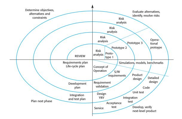
Figure 4.5 Boehm's spiral model of the software process (©IEEE, 1988) something that can go wrong. For example, if the intention is to use a new programming language, a risk is that the available compilers are unreliable or do not produce sufficiently efficient object code. Risks result in project problems such as schedule and cost overrun so risk minimisation is a very important project management activity. Risk management, an essential part of project management, is covered in Chapter 5.
