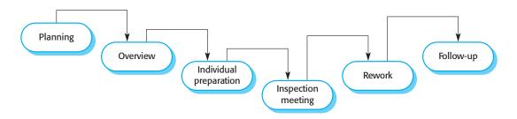
Figure 22.6 The inspection process
