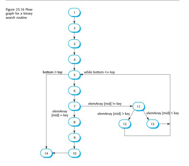
The flow graph for the binary search procedure is shown in Figure 23.16 where each node represents a line in the program with an executable statement. By tracing the flow, therefore, you can see that the paths through the binary search flow graph are:
