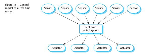
handled by the system. This sensor-system-actuator model of an embedded realtime system is illustrated in Figure 15.1.
