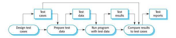
Figure 23.2 A model of the software testing process defects. The test cases can be deliberately obscure and need not reflect how the system is normally used. For validation testing, a successful test is one where the system performs correctly. For defect testing, a successful test is one that exposes a defect that causes the system to perform incorrectly.
