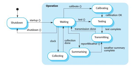
Figure 14.14 State diagram for WeatherStation
