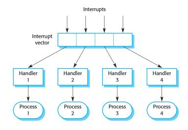
An interrupt-driven control model is illustrated in Figure 11.10. There are a known number of interrupt types with a handler defined for each type. Each type of interrupt is associated with the memory location where its handler's address is stored. When an interrupt of a particular type is received, a hardware switch causes control to be transferred immediately to its handler. This interrupt handler may then start or stop other processes in response to the event signalled by the interrupt.
