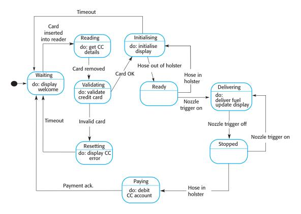
Figure 15.3 State machine model of a petrol (gas) pump
