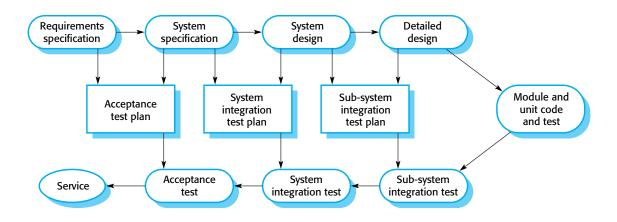
Figure 4.10 Testing phases in the software process Normally, component development and testing are interleaved. Programmers make up their own test data and incrementally test the code as it is developed. This is an economically sensible approach, as the programmer knows the component best and is therefore the best person to generate test cases.
