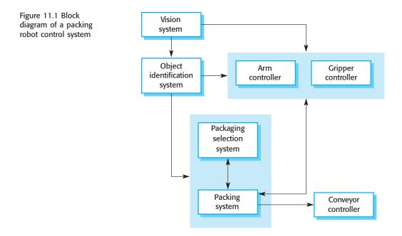
objects on a conveyor, identify the type of object and select the right kind of packaging. The system then moves objects from the delivery conveyor to be packaged. It places packaged objects on another conveyor. Other examples of architectural designs at this level are shown in Chapter 2 (Figures 2.6 and 2.8).
