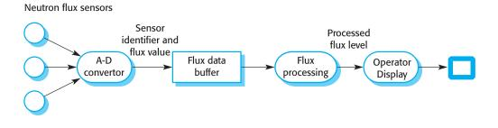
Figure 15.12 Neutron flux data acquisition
