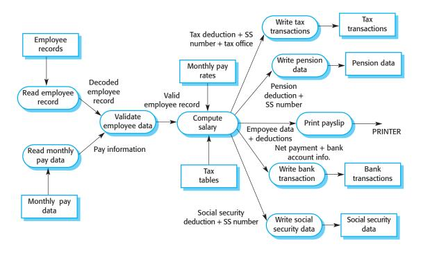
Figure 13.2 Dataflow diagram of a payroll system payments are made. You can see how this system follows the basic input-processoutput structure:
