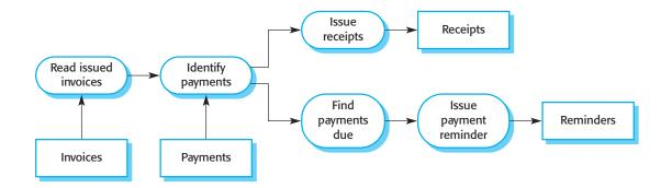
Figure 11.6 A pipeline model of an invoice processing system made are reconciled with the invoices. For those invoices that have been paid, a receipt is issued. For those invoices that have not been paid within the allowed payment time, a reminder is issued.
