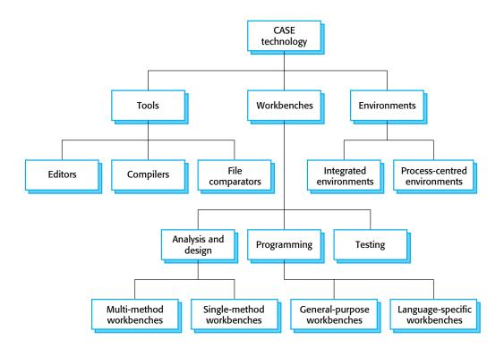
Figure 4.16 Tools, workbenches and environments
