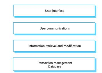
Figure 13.6 A layered model of an information system
