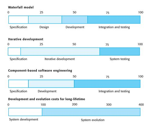
Figure 1.2 Software engineering activity cost distribution each of the different generic approaches to software development has a different profile of cost distribution across the software process activities. If you assume that the total cost of developing a complex software system is 100 cost units then Figure 1.2 illustrates how these are spent on different process activities.
